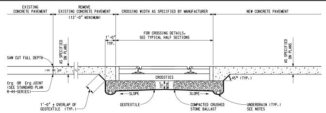
TRACK CROSSING, DETAIL 1 (EXISTING CONCRETE PAVEMENT SHOWN)
