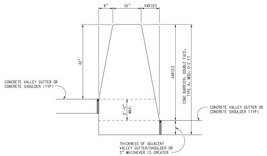
CONCRETE BARRIER, TYPE A WITH
