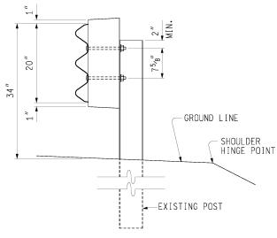
NOTE: HOLES IN STEEL POST SHALL BE DRILLED NOT BURNED.
