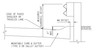
\*\* 2" WHEN CURB IS PLACED NEXT TO SHOULDER 10" WHEN CURB IS PLACED NEXT TO TRAVELED LANE
