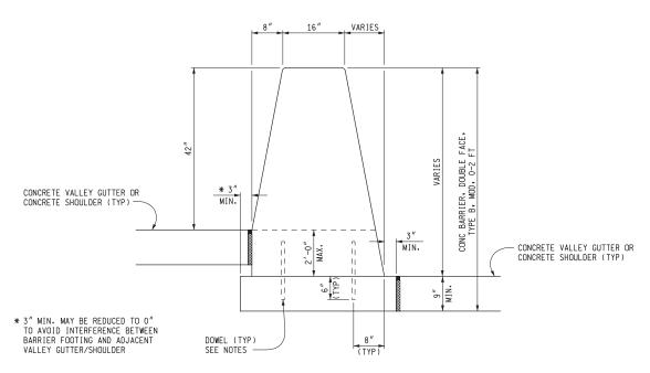
CONCRETE BARRIER, TYPE B WITH HEIGHT DIFFERENCE BETWEEN MEDIAN SHOULDERS  $_{(2'-0'' \text{ MAXIMUM})}$
