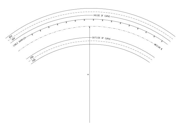
RECOMMENDED CABLE BARRIER PLACEMENT ON CURVED ROADWAYS  $5.730' \le R \le 11.460'$  R < 5.730' WITH EQUAL EMBANKMENT HEIGHT AND 1:4 OR FLATTER MEDIAN SLOPES
