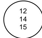
(Where the sampler is driven distances other than 18", the distance is shown in the circle with the number of blows in the form of a fraction.) [Indicate actual hammer type used] (4-19-2021)
