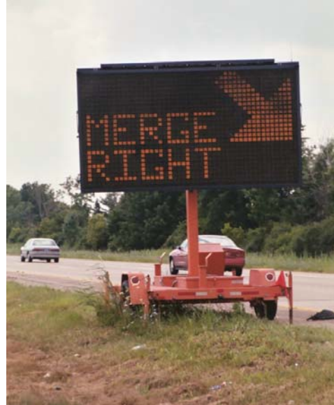
Photograph 3. Changeable Message Sign - Phase II (2003 Construction Season)
