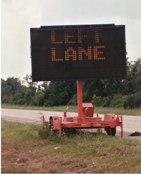
Photograph 2. Changeable Message Sign - Phase I (2003 Construction Season)
