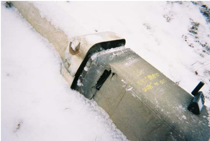
Figure 7. Breakaway light standard struck by vehicle.
