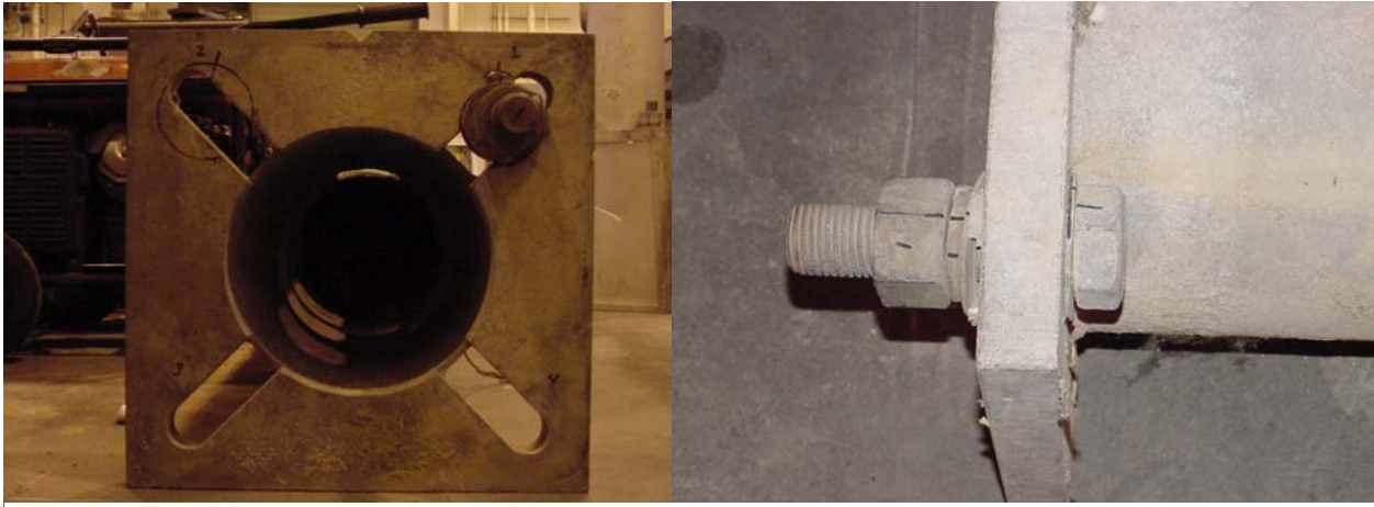
Figure 18. Steel screw-in foundation. Note the open slots used to accommodate variable bolt circle sizes.
