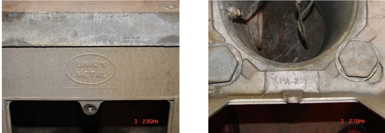
Figure 15. Die stamp APA 2852. The 52 is not legible due to die stamp imperfection.
