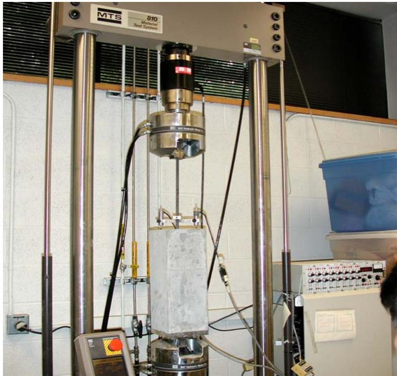
Figure 7.3 Pullout test setup
