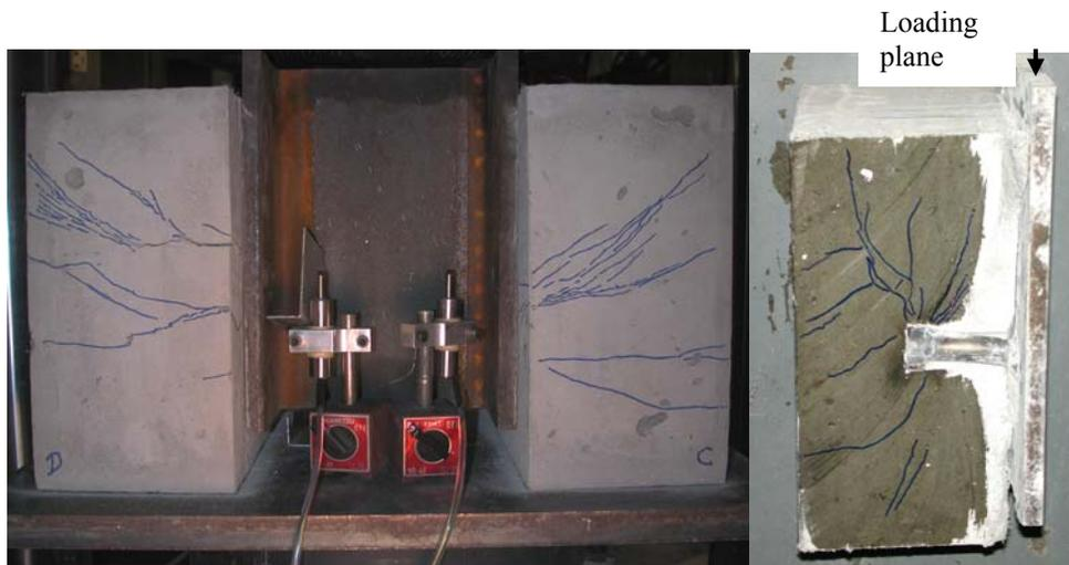
Figure 7.13 Microcracks developed outside (left) and inside (right, cut section along shear stud) of ECC specimen
