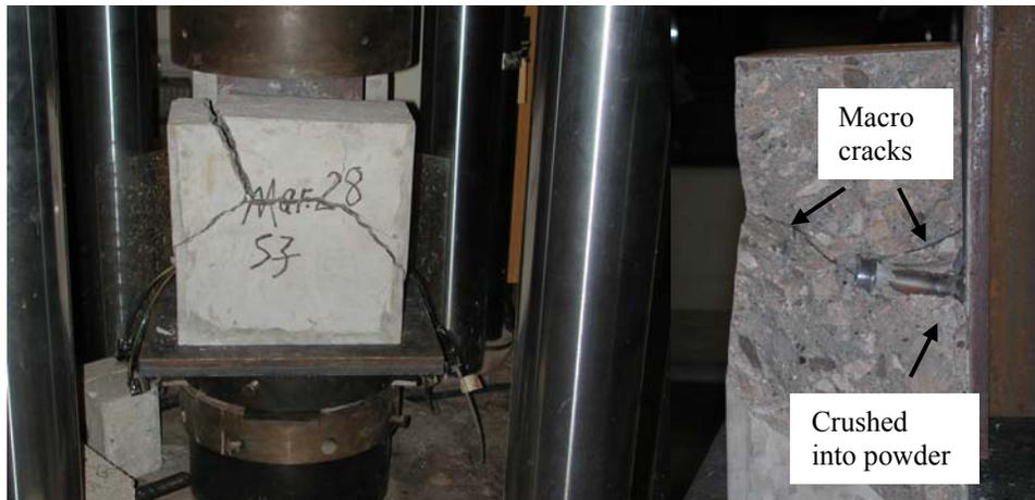
Figure 7.12 Macro cracks developed in concrete pushout specimen show a brittle failure mode
