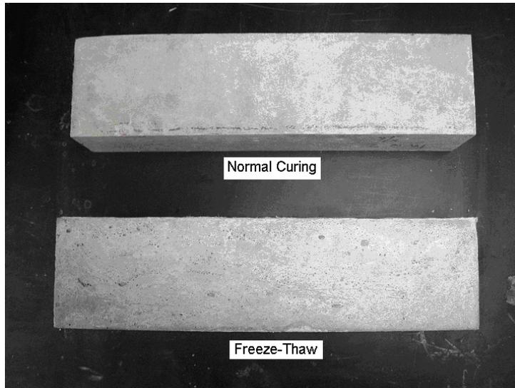
Figure 5.4. M34 ECC Normal Curing and Freeze-Thaw Specimens
