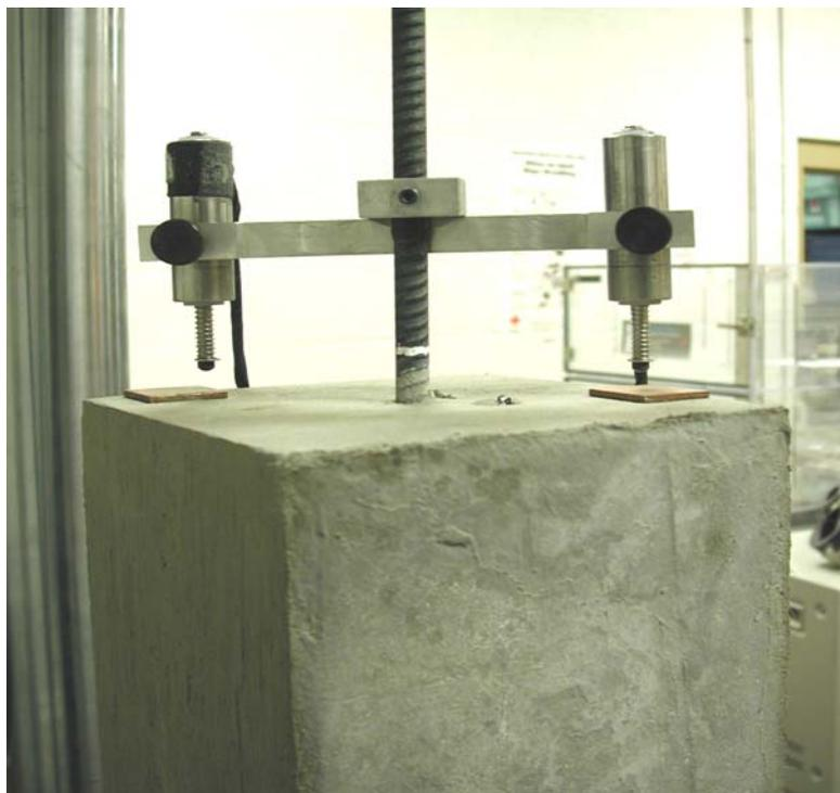
Figure 7.4 LVDTs attached to the reinforcement for measurement of pullout displacement
