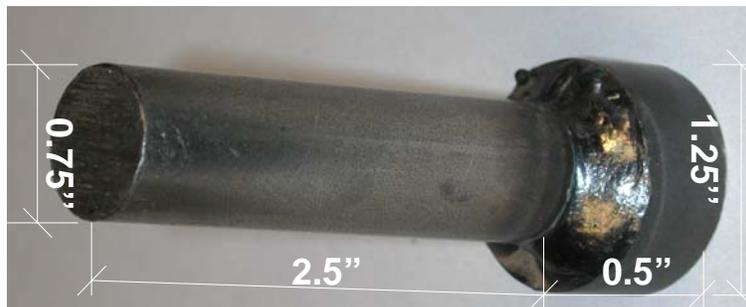
Figure 7.8 Geometry of a shear stud
