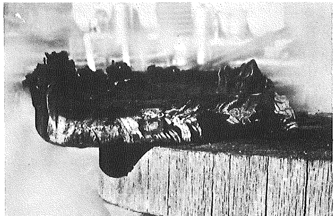
Figure 20. Single-acting diesel McKiernan-Terrys DE-30 and DE-40. Oak cushion block is shown before driving at lower left, resting on driving cap. At lower right, a section of a similar block is shown after hard driving, resting on an unused block.
