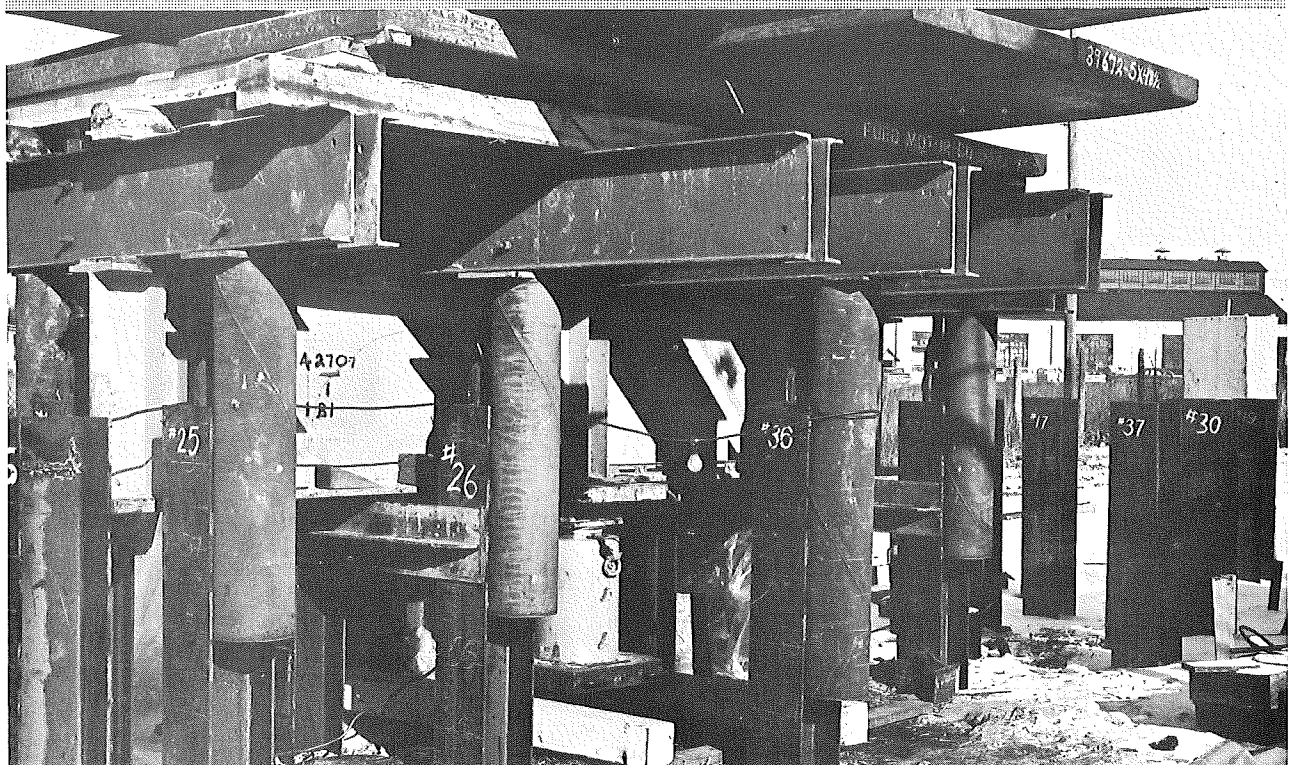
Figure 102. Belleville load reaction assembly, showing reaction frame with 100 tons of steel slabs in place (top), and reaction beam and jack in place (bottom). Note spacing of reaction piles.
