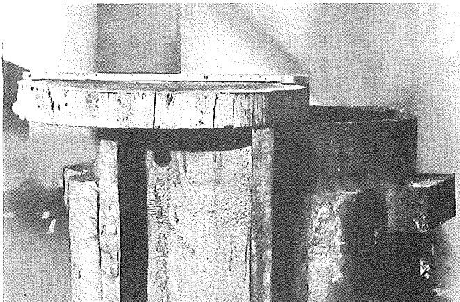
Figure 20. Single-acting diesel McKiernan-Terrys DE-30 and DE-40. Oak cushion block is shown before driving at lower left, resting on driving cap. At lower right, a section of a similar block is shown after hard driving, resting on an unused block.
