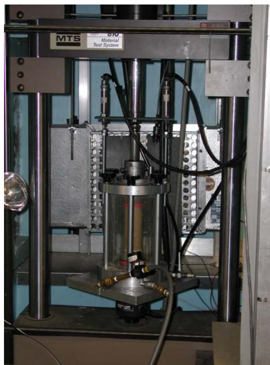
Figure 3.8 Cyclic load test setup
