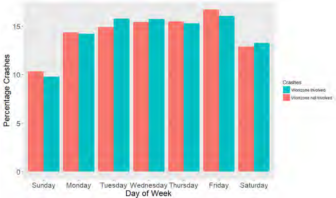
Figure 6. Percentage Distribution across Days of the Week for Work zone and Non-work zone Crashes (2015-2016)
