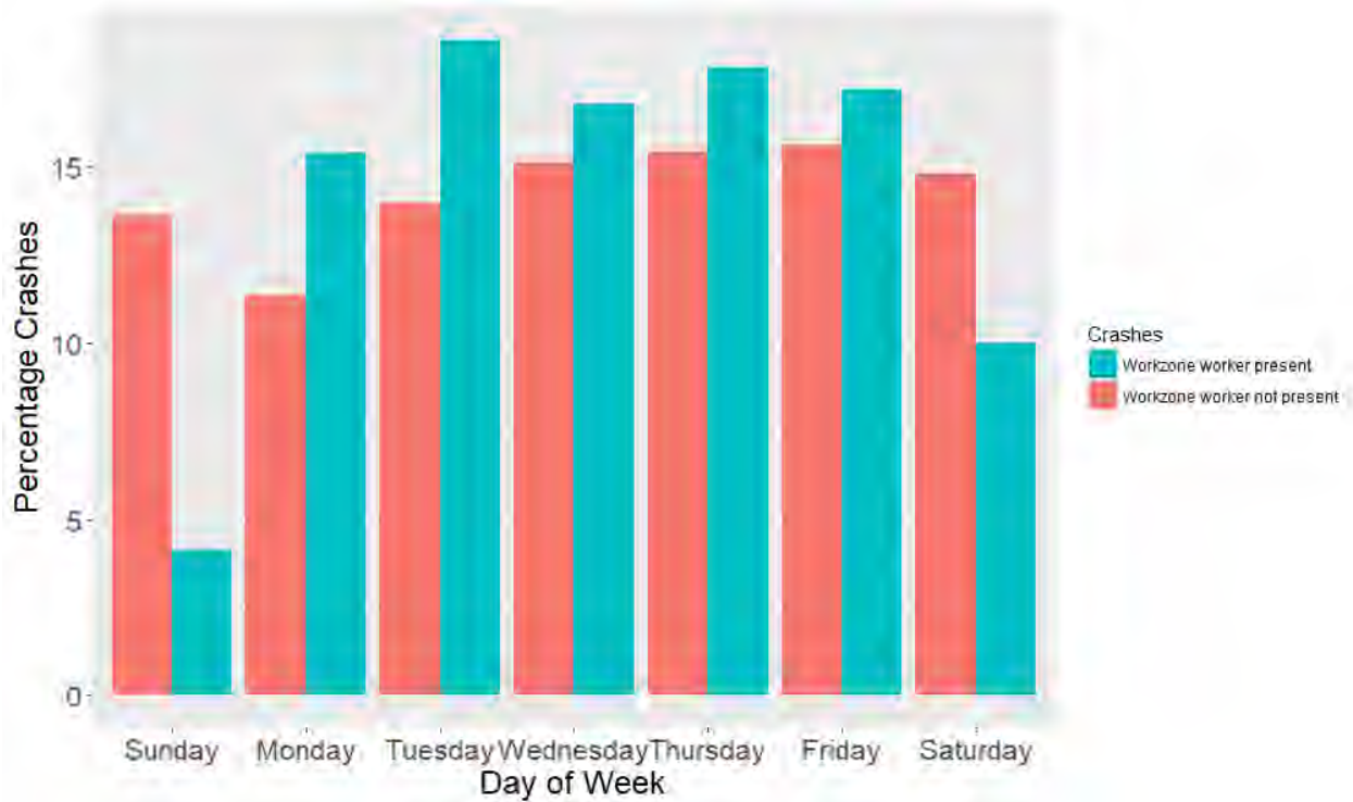
Figure 7. Percentage Distribution Across Days of the Week for Crashes in Work zones with and without Workers Present (2015-2016)
