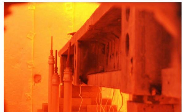
Concrete beams prestressed with CFRP strands were subjected to fire/loading tests to evaluate their fire endurance.
