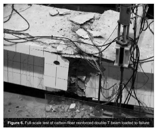
1.4 times the service load. Researchers observed significant cracking before failure load was reached, which gives the desired indicator of possible failure before it occurs (Figure 6). The beam test results supported design expectations, allowing bridge construction to commence.
