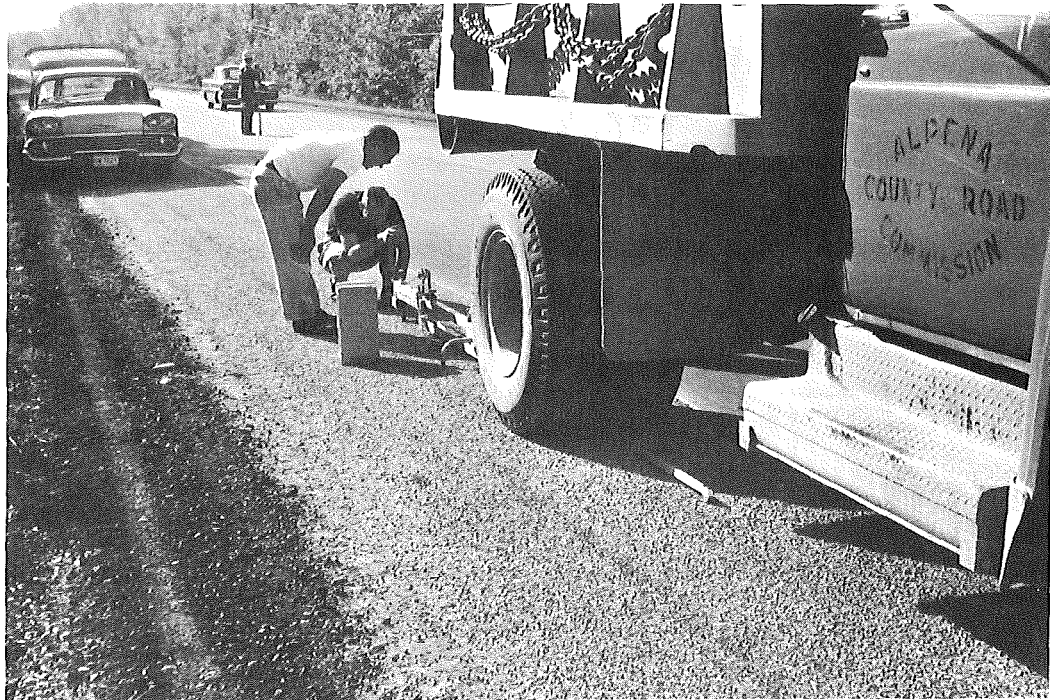
Figure 16. Benkelman beam measuring surface movement under dual wheel load.
