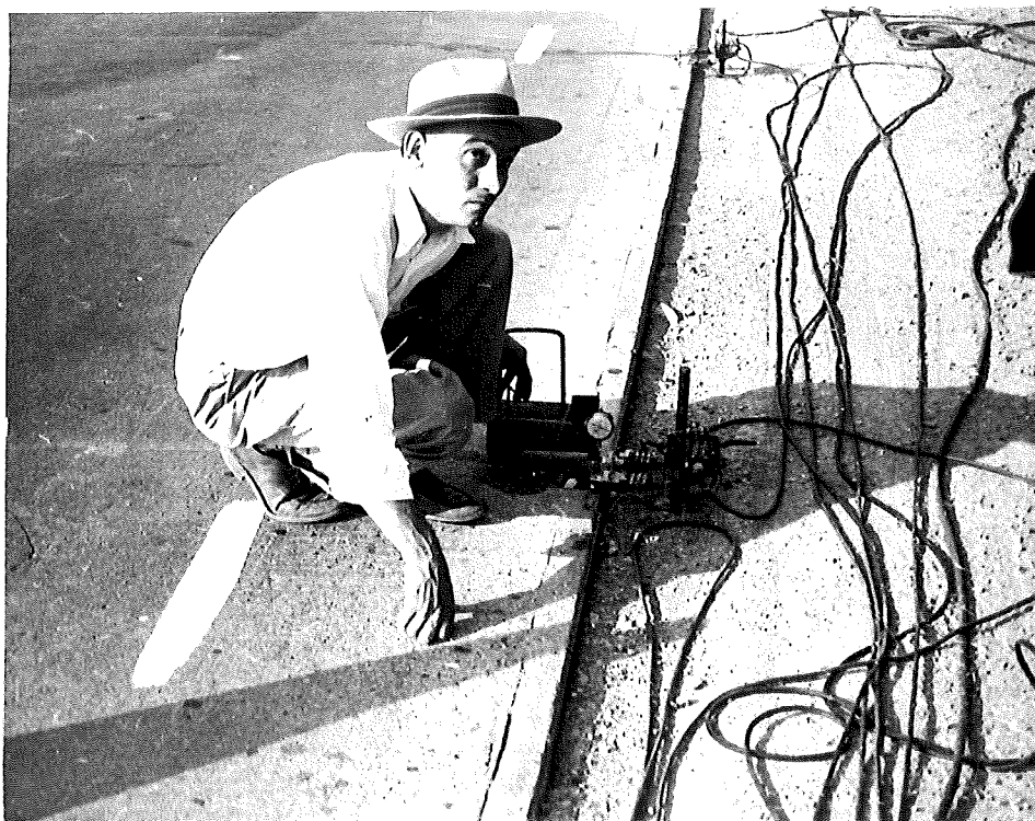
FIGURE 3. CALIBRATION OF DEFLECTOMETERS IN THE FIELD BY A MECHANICAL CALIBRATOR CONSTRUCTED BY THE LABORATORY.
