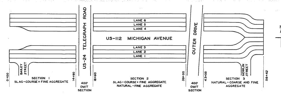
NOTE: IN EVERY CASE WHEEL TRACK I IS THE SOUTH TRACK OF A LANE AND WHEEL TRACK 2 IS THE NORTH TRACK. OUTSIDE LANES ARE NOT INCLUDED IN TEST RUNS BECAUSE OF PARKED CARS.
