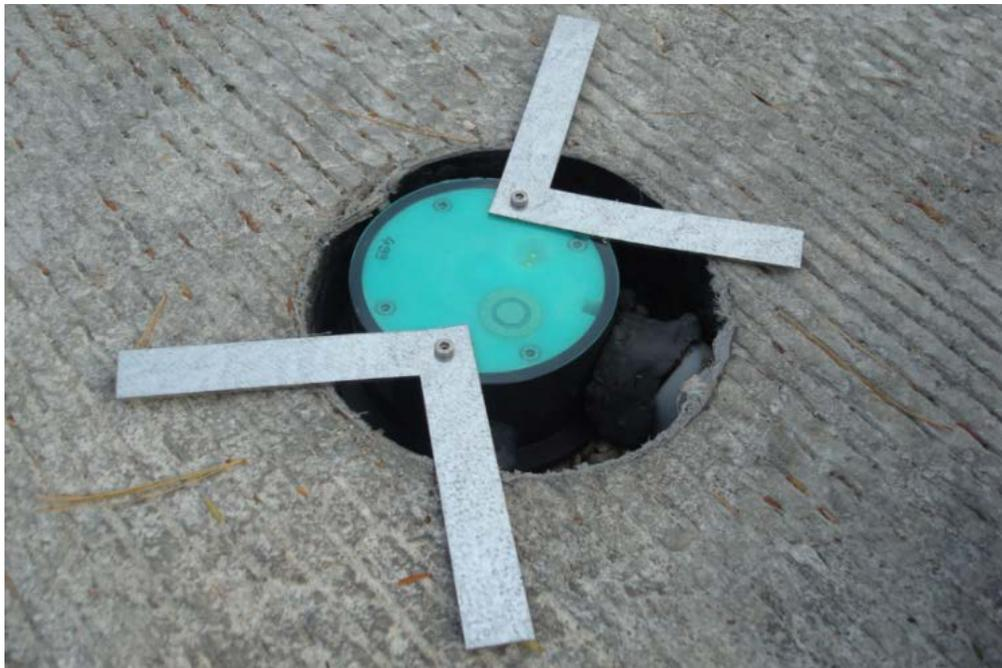
Figure 20: Lufft Intelligent Road Sensor
