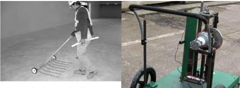
Researchers aimed to replace traditional tests of bridge deck subsurface damage (such as the chain drag test above) with a system that electronically interprets sound readings (an early prototype is shown at right).
