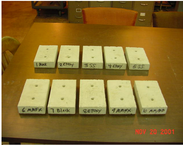
Figure 3 Concrete blocks with #4 bars embedded with 1/2 in cover, before testing (above), and after 1,184 days (above right). Note the corrosion staining in specimen 1 (uncoated bar) in top row, left block of right photo.
