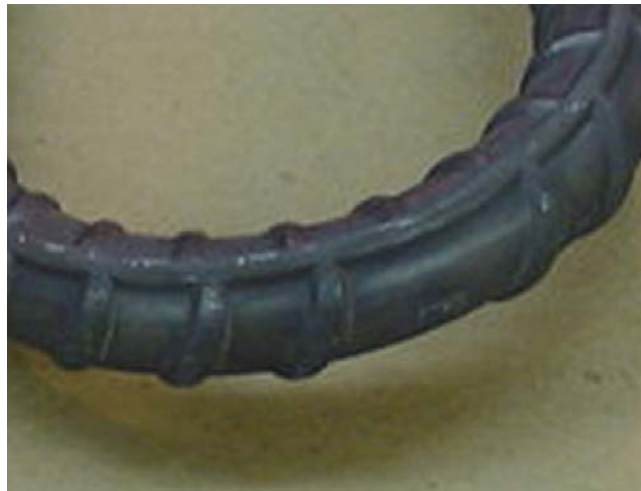
Figure 1 MMFX Bend Specimen, #4 bar
