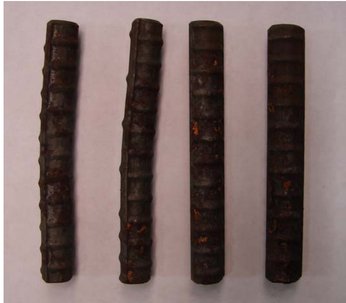
Figure 4 Uncoated reinforcement removed from concrete blocks. Note the general corrosion on all samples.
