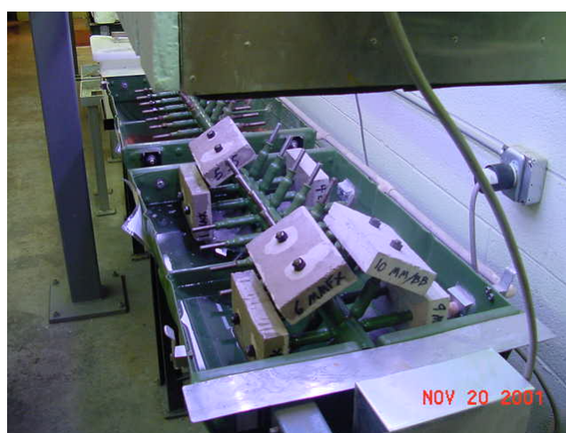
Figure 2 Corrosion tank with cover raised
