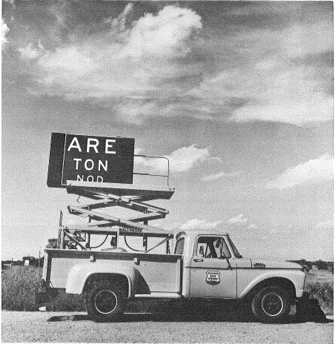
Figure 2. Illuminated case sign mounted on lift platform for night testing.
