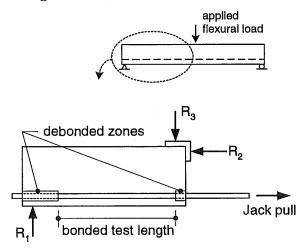
Figure 2-7: Semi-Beam Test Specimen
