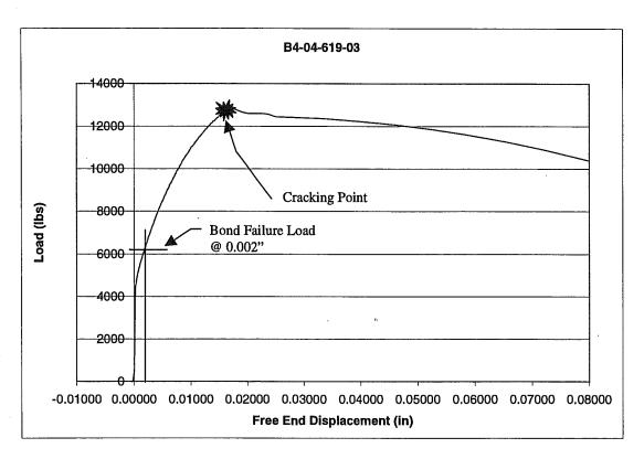
Figure 4-3: Load-Displacement Curve for B4-04-619-03, Extended Scale
