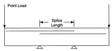
Figure 2-6: Lap-Splice Test
