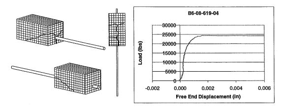
Figure 4-5: Crack Pattern and Load-Displacement for Specimen B6-08-619-04 (Bond Failure)
