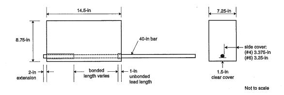
Figure 3-3: Debond Schematic with Specimen Dimensions
