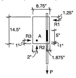
Figure 4-8: Reaction Locations for Sample Calculation for Specimen B6-05-619-01
