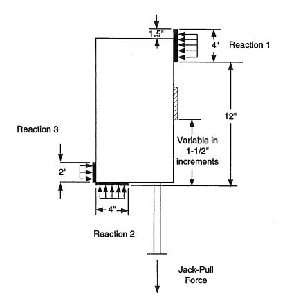
Figure 3-6: Reactions on Specimen
