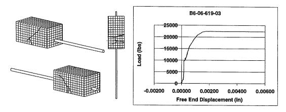
Figure 4-6: Crack Pattern and Load-Displacement for Specimen B6-08-619-03 (Flexure Failure)
