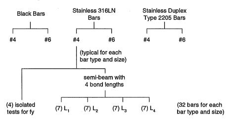
Figure 1-2: Number of Semi-beam Bond Specimens
