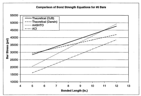
Figure 4-2: Comparison of Bond Strength Equations for No. 6 Bars
