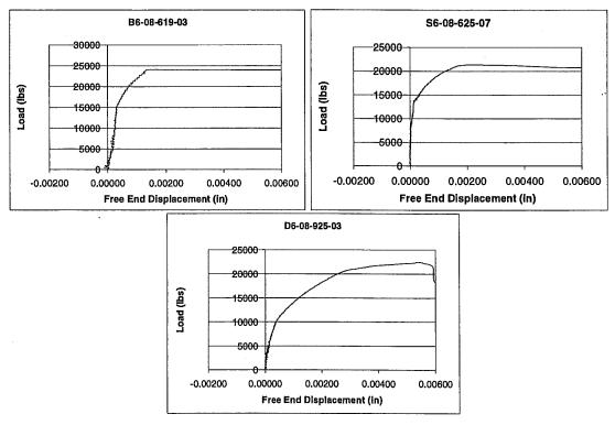
Figure 4-17: Comparison of Load-Displacement Plots for Specimens B6-08-619-03, S6-08-625-07, and D6-08-925-03
