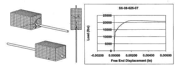
Figure 4-11: Crack Pattern and Load-Displacement Curve for Specimen S6-08-625-07
