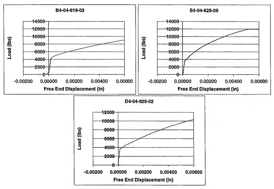
Figure 4-14: Comparison of Load-Displacement Plots for Specimens B4-04-619-03, S4-04-625-05 and D4-04-925-02
