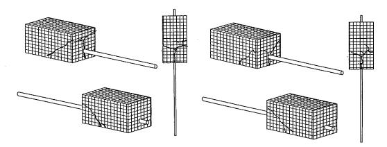
Figure 4-15: Comparison of Crack Patterns for B4-04-619-03 and S4-04-625-06
