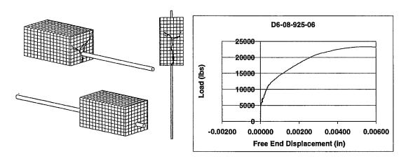
Figure 4-13: Crack Pattern and Load-Displacement Curve for Specimen D6-08-925-06
