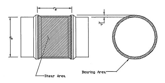
Figure 2-1: Relative Rib Area Diagram
