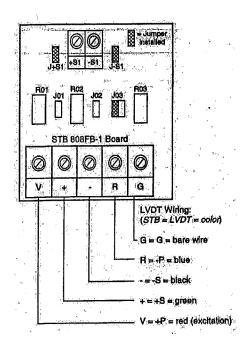
Figure E-3: Wiring Schematic for LVDT Connection to 808FB-1 Terminal Board
