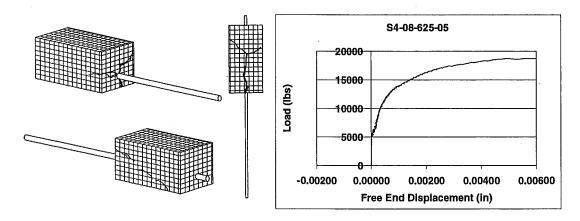
Figure 4-10: Crack Pattern and Load-Displacement Curve for Specimen S4-08-625-05
