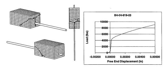
Figure 4-4: Crack Pattern and Load-Displacement for Specimen B4-04-619-03
