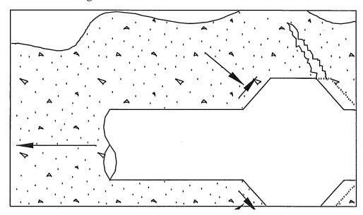
Figure 1-1: Step 2, Microcrack Formation
