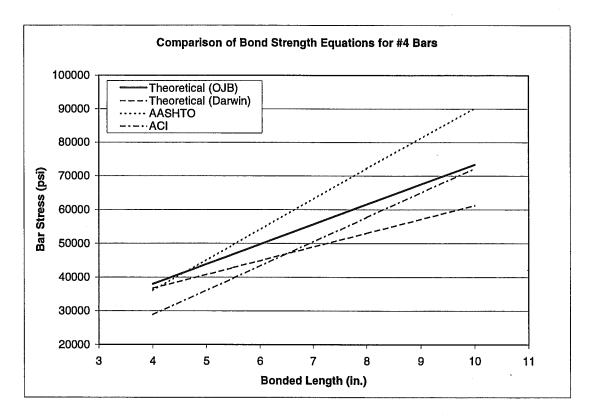
Figure 4-1: Comparison of Bond Strength Equations for No. 4 Bars
