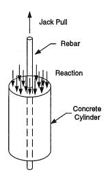
Figure 2-3: Pullout Test
