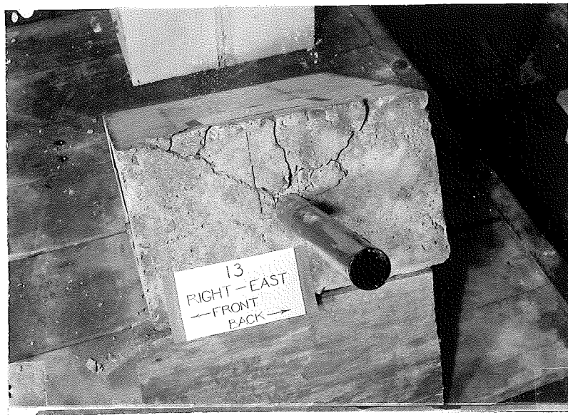
Figure 10. Typical failure of 1-1/4 inch dowel.
