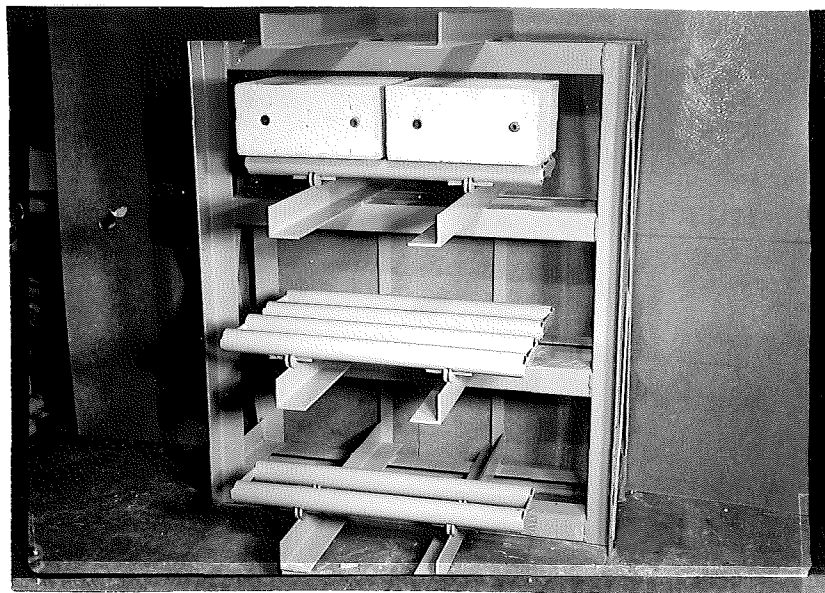
Figure 5. Method of storing specimen during curing period.
