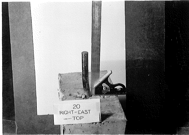
Figure 9. Typical failure of 3/4 inch dowel.
