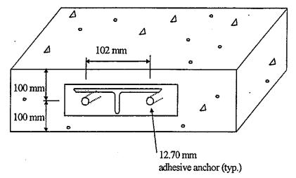
Embedment Depth = 110 mm (*Hilti HY-150*) Host concrete f<sup>°</sup>c = 28 MPa A 248MPa threaded rod; f<sup>°</sup>y=250 MPa ;  $f_{ult}$ =420 MPa Tensile Area of 12.70 mm threaded rod = 92 mm<sup>2</sup>
