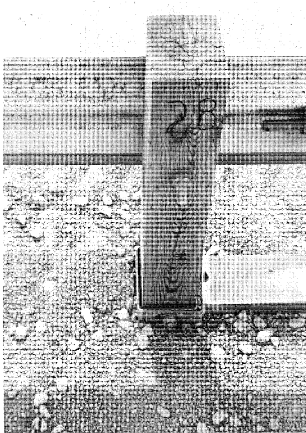
Figure 24. Permanent Set Deflections of End Anchorages, Test MIW-1
