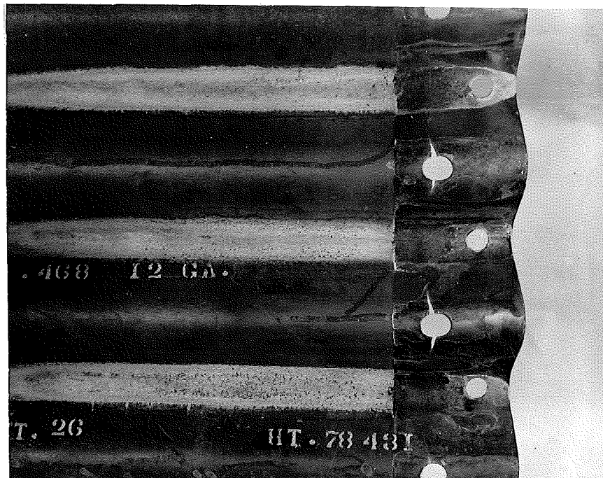
Figure 6. Showing condition of plate at bolt holes. Half of specimen illustrated in Figure 5.
