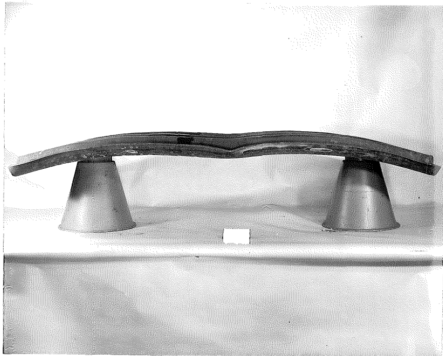
Figure 10. Typical failure of plain beam specimen, 50 inch radius, 7 gage.
