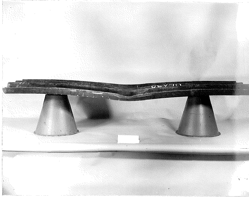
Figure 9. Typical failure of plain beam specimen, 150 inch radius, 7 gage.
