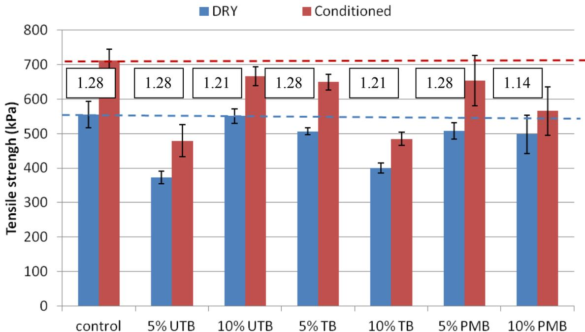
**Figure 6-9: Indirect tensile strength results for dry and conditioned asphalt mixtures**
