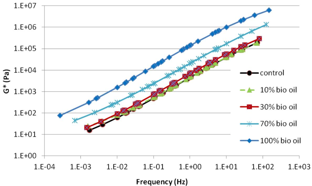
**Figure 5-13: Master curve plot for RTFO aged samples of control binder, 10%, 30%, 70% and 100% bio oil blended asphalt binders**
