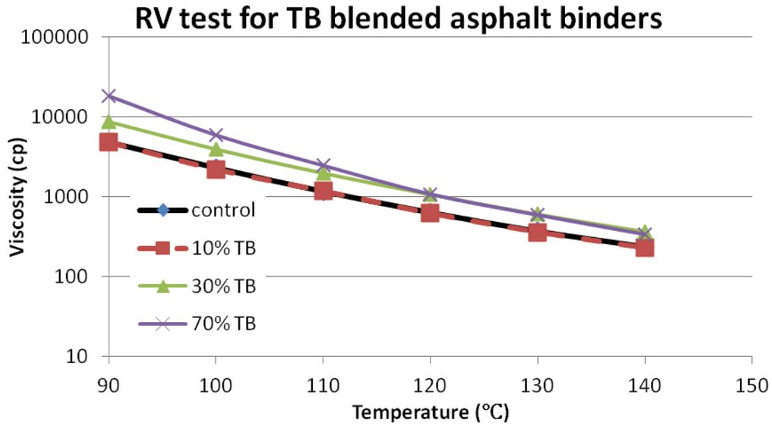
**Figure 5-5:RV results for control asphalt binder PG 58-28, and 10%, 30%, 70% and 100% TB bioasphalt binders**
