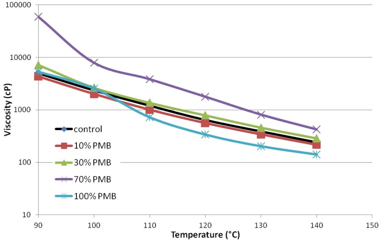
**Figure 5-3: RV results for control asphalt binder, 10%, 30%, 70% and 100% PMB bioasphalt binders**
