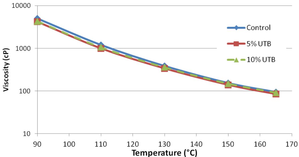
**Figure 4-1: RV test results for control binder, 5%, 10% and 100% UTB modified asphalt binders before RTFO aging**
