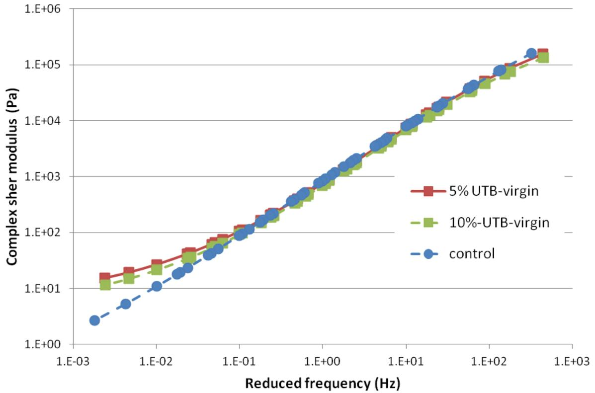
**Figure 4-8:  $G^*$  master curve plot for control binder, 5% and 10% UTB modified asphalt binders before RTFO aging**
