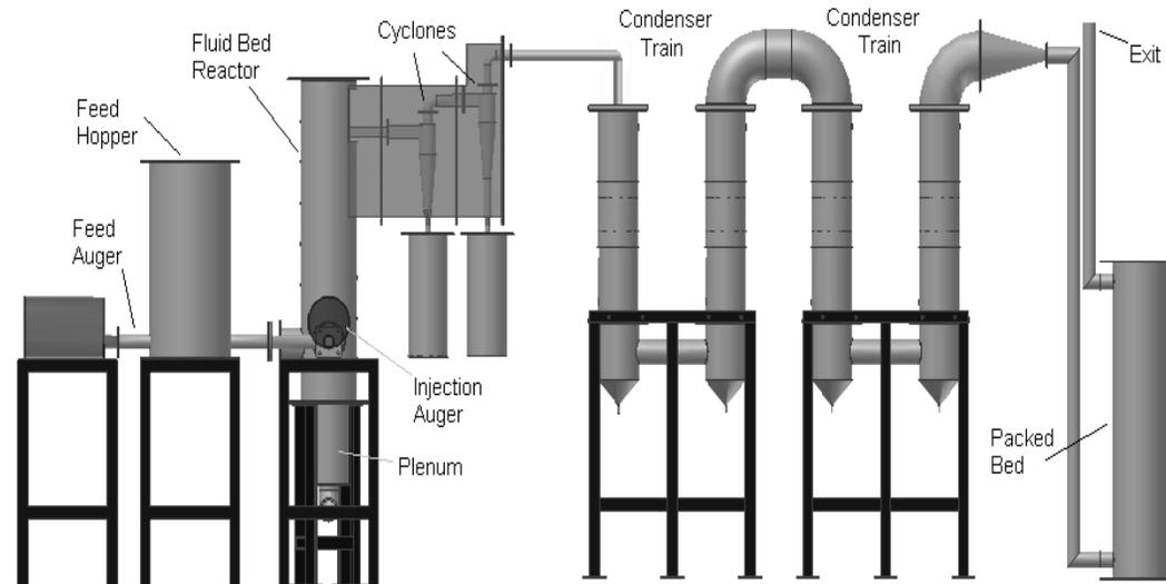
**Figure 2-1: A schematic of the fluidized bed fast pyrolysis unit used in this research**
