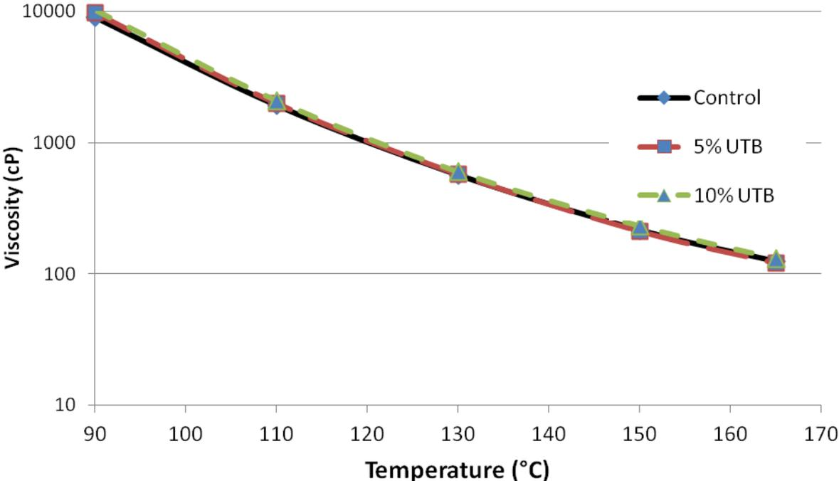
**Figure 4-4: RV test results of control binder, 5%, and 10% UTB modified binders, after RTFO aging**
