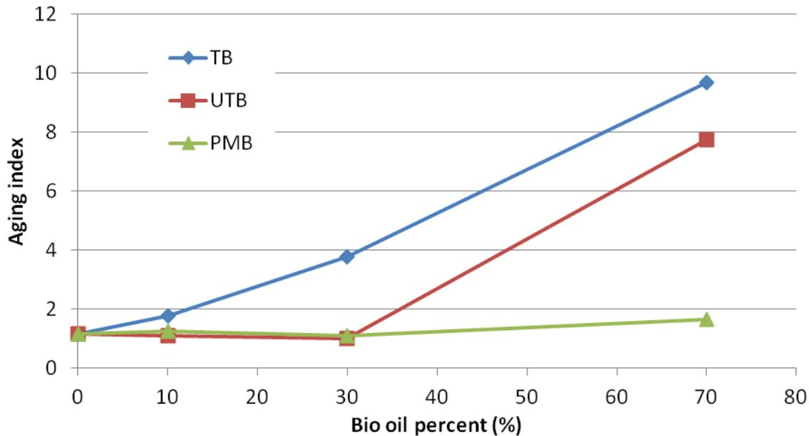
**Figure 5-15: Aging indexes of control binder, 10%, 30% and 70% bioasphalt binders after RTFO aging in temperature range of 40°C to 70°C**
