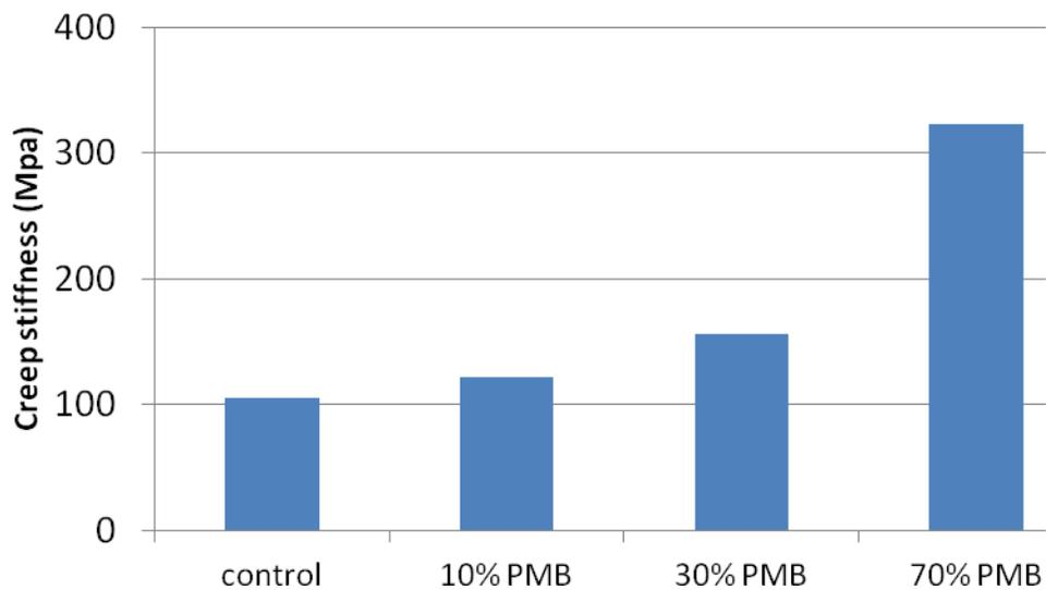
**Figure 5-20: Creep stiffness of control binder, 10%, 30% and 70% PMB bioasphalt at 60s during BBR test**
