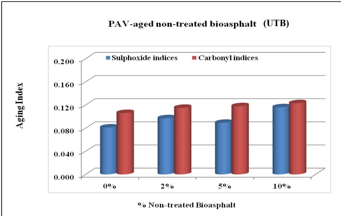
**Figure 3-9: Bar chart of aging indices for PAV-aged control and untreated bioasphalt**
