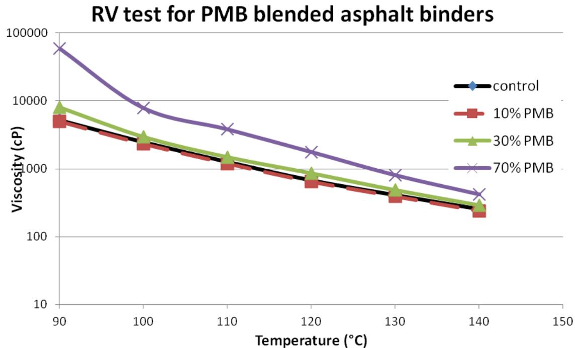
**Figure 5-6: RV results for control asphalt binder PG 58-28, and 10%, 30%, 70% and 100% PMB bioasphalt binders**
