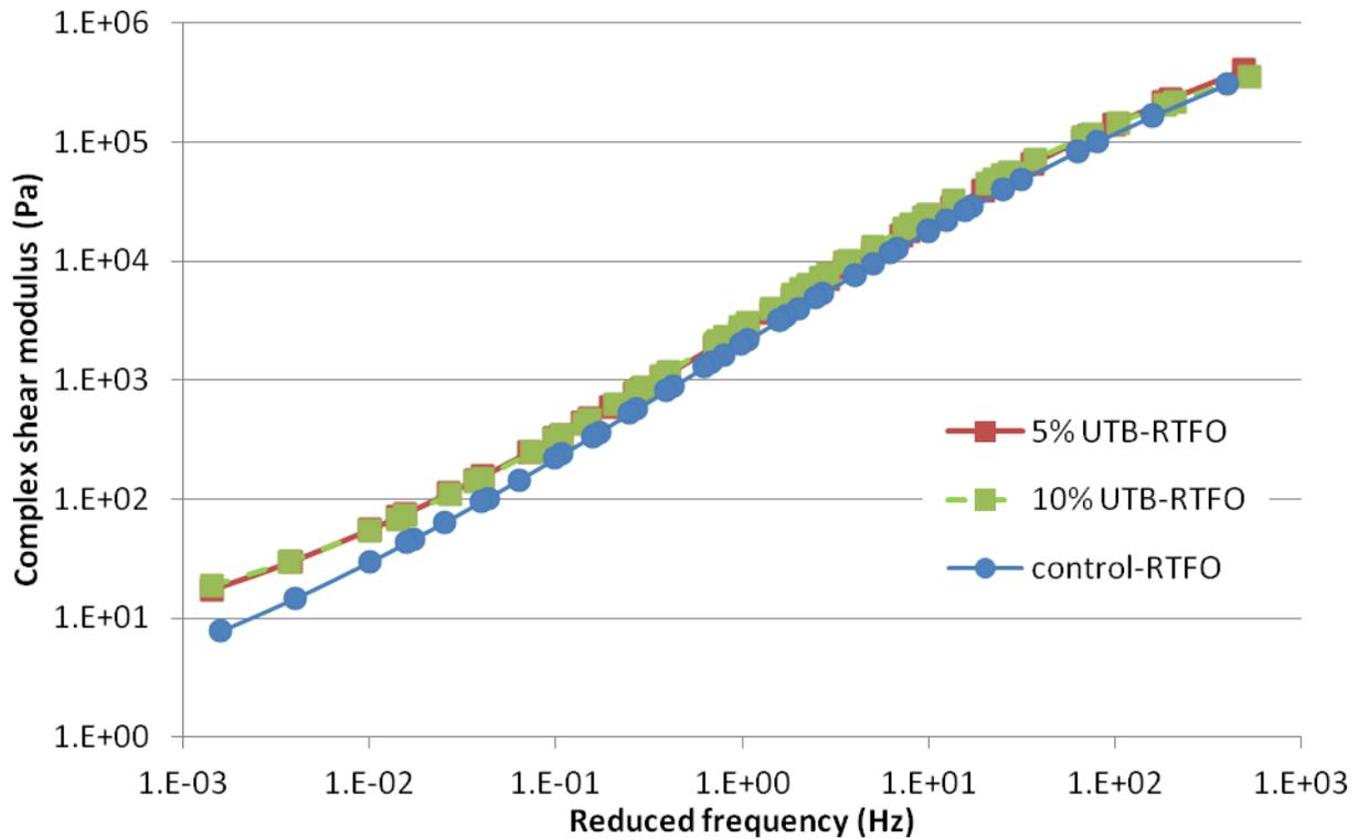
**Figure 4-11:  $G^*$  master curve plot for control binder, 5% and 10% UTB modified asphalt binders after RTFO aging**
