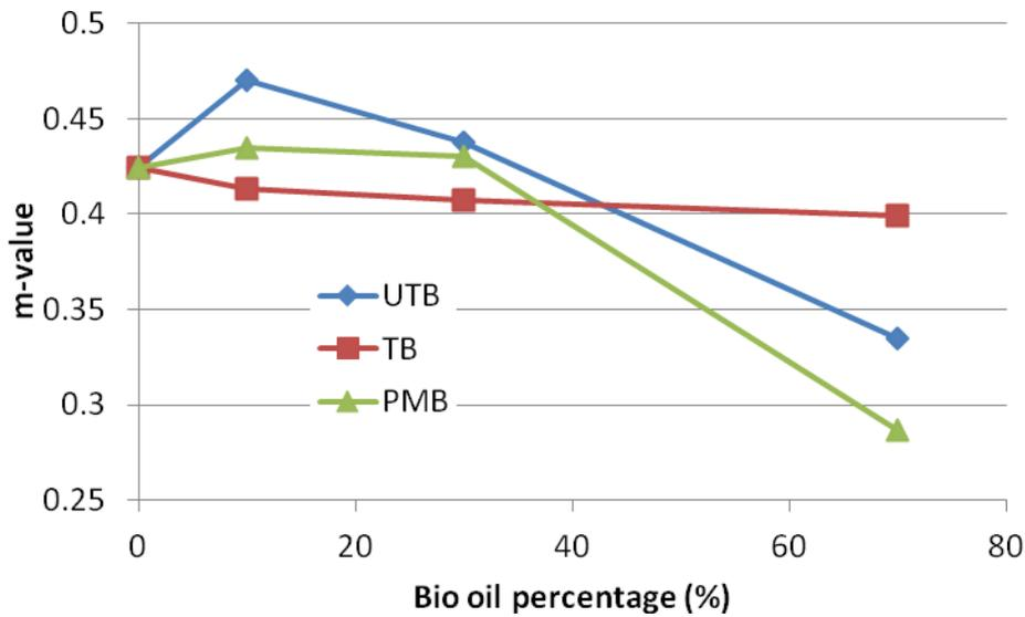
**Figure 5-23: Comparison of the m-value of three types of bioasphalt binder at 60s**
