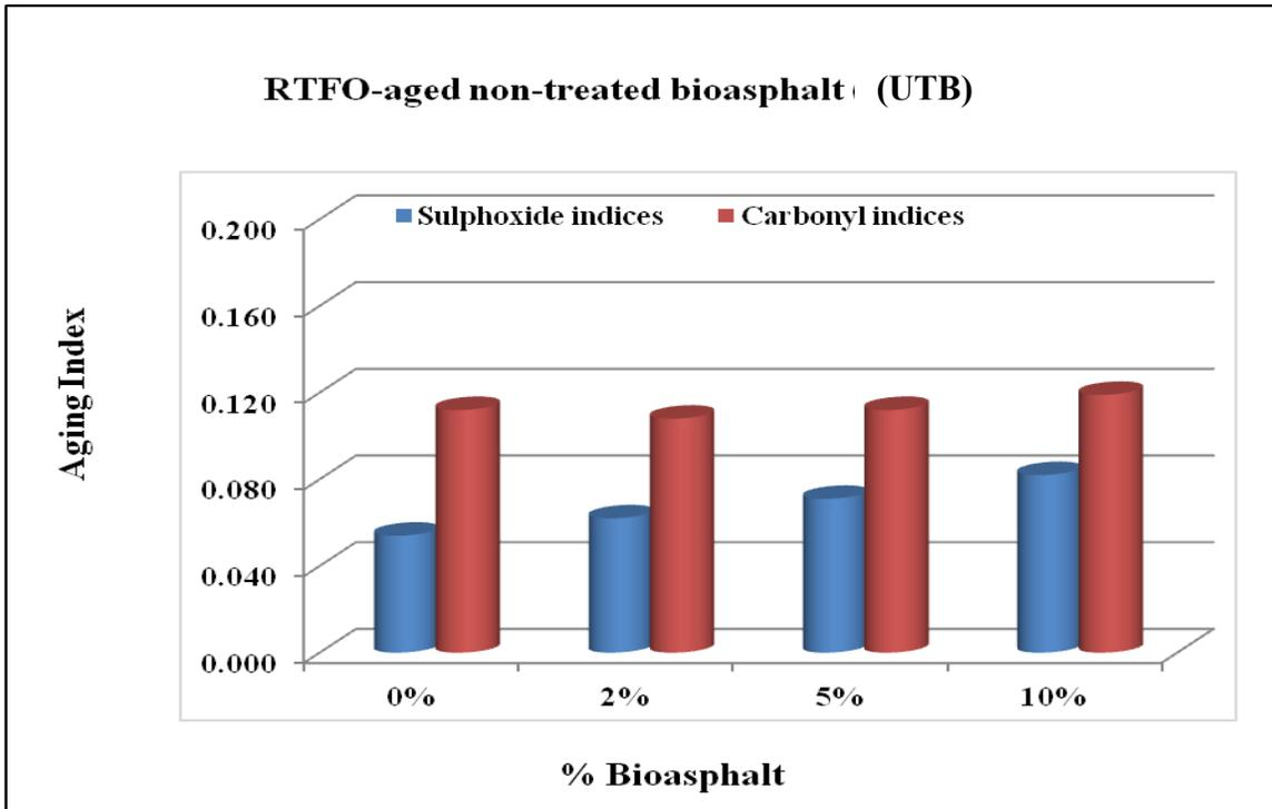
Figure 3-7: Bar chart of aging indices for RTFO-aged control and untreated bioasphalt
