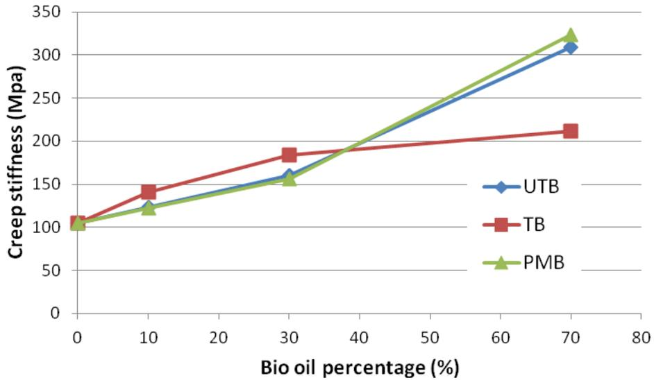
**Figure 5-22: Comparison of the creep stiffness of three types of bioasphalt binder at 60s**
