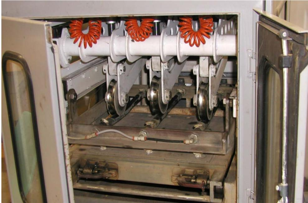
**Figure 6-5: Set-up of the Asphalt Pavement Analyzer for rutting performance**
