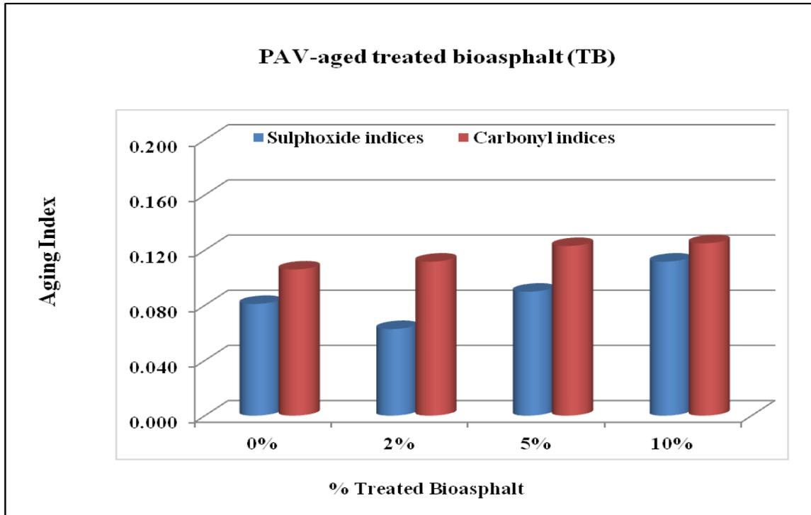
Figure 3-10: Bar chart of aging indices for PAV-aged control and treated bioasphalt
