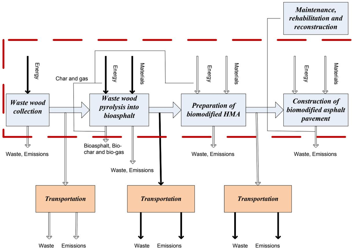
**Figure 7-1: Inventory for the bioasphalt production and construction of bio oil modified asphalt pavements**
