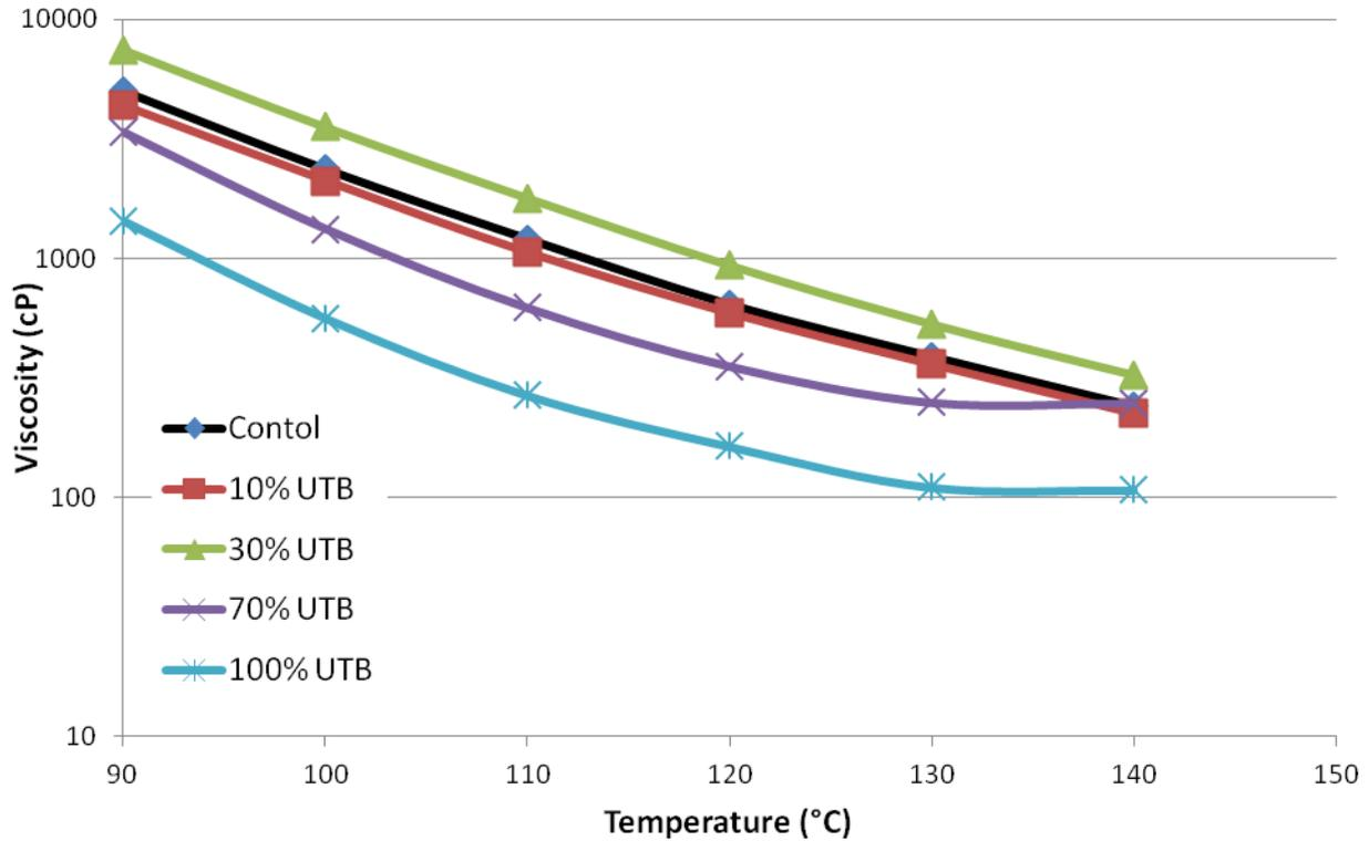
**Figure 5-1: RV test results for control binder, 10%, 30%, 70% and 100% UTB bioasphalt binders**
