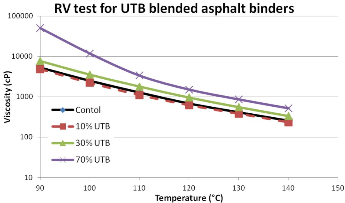
**Figure 5-4: RV results for control asphalt binder PG 58-28, and 10%, 30%, 70% and 100% UTB bioasphalt binders after RTFO aging**
