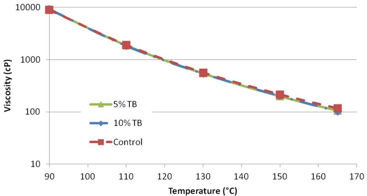
**Figure 4-6: RV test results of control binder, 5%, and 10% UTB modified binders, after RTFO aging**
