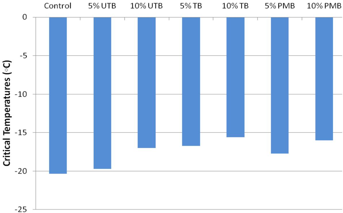
**Figure 4-19: Critical low temperatures of control binder and the three types of bio oil modified asphalt binders obtained from BBR test**
