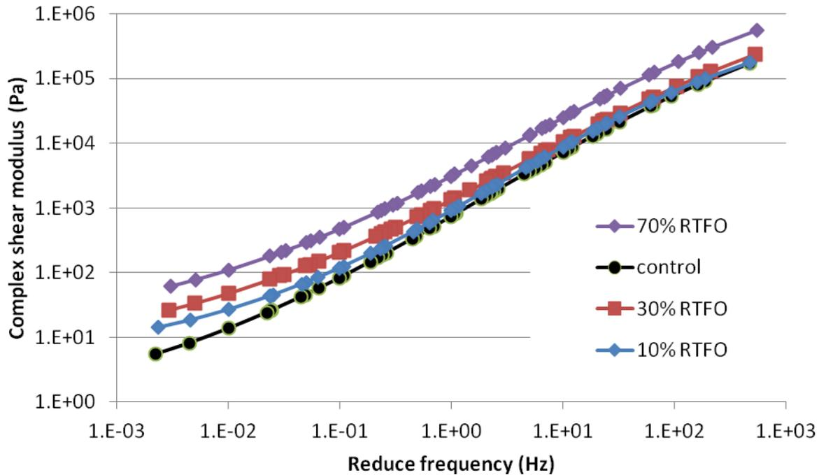
**Figure 5-14: Master curve plot for control binder, 10%, 30% and 70% PMB bioasphalt binders after RTFO aging**
