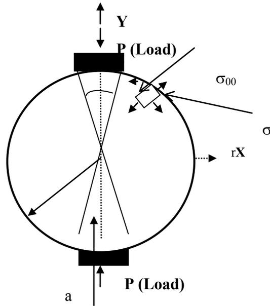
**Figure 6-8: Schematic of the indirect tensile strength test for moisture susceptibility**
