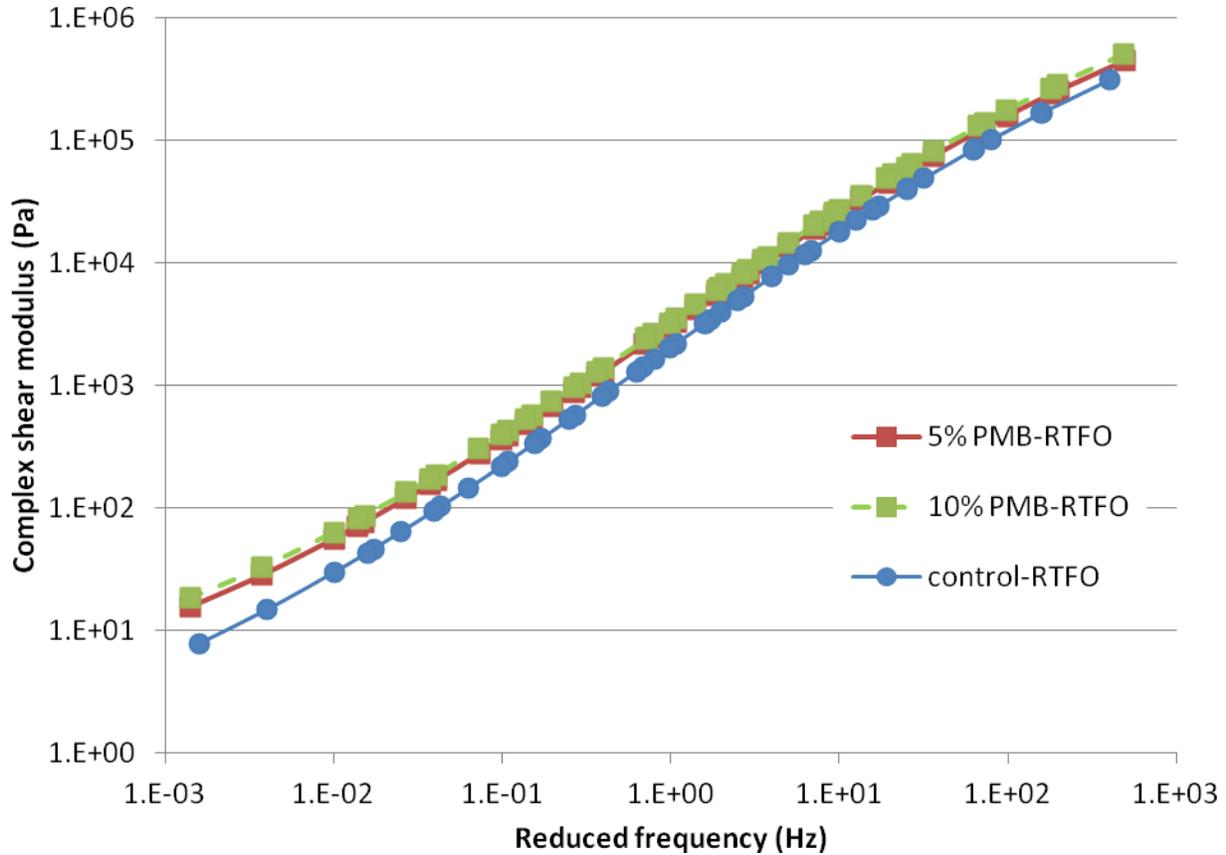
**Figure 4-13: G\* master curve plot for control binder, 5% and 10% PMB modified asphalt binders after RTFO aging**
