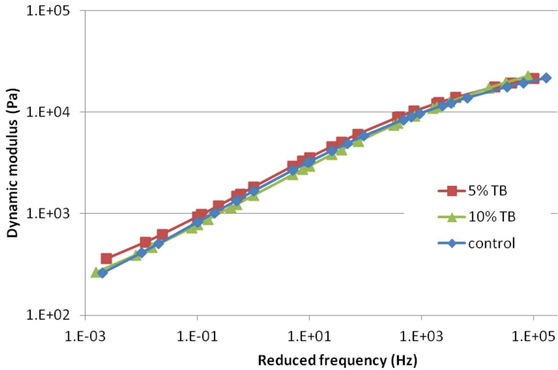
**Figure 6-3: Dynamic modulus master curve plot for control asphalt mixture, 5% and 10% TB modified asphalt mixture**
