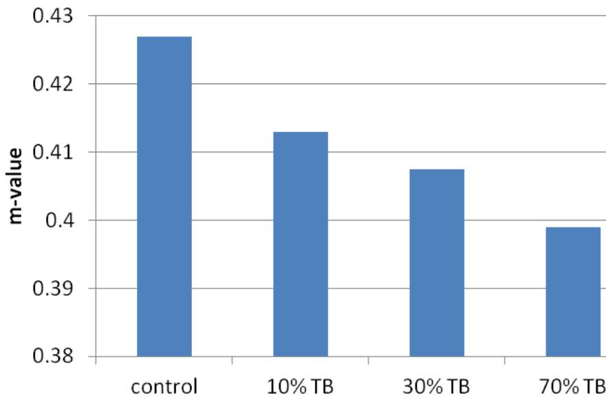
**Figure 5-19: M-value of control binder, 10%, 30% and 70% TB bioasphalt at 60s in BBR test**
