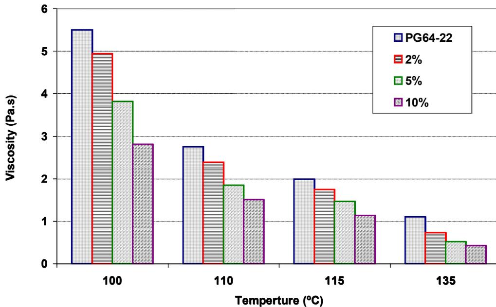
**Figure 1-3: Effect of swine waste binder on petroleum-based asphalt (Fini 2010)**
