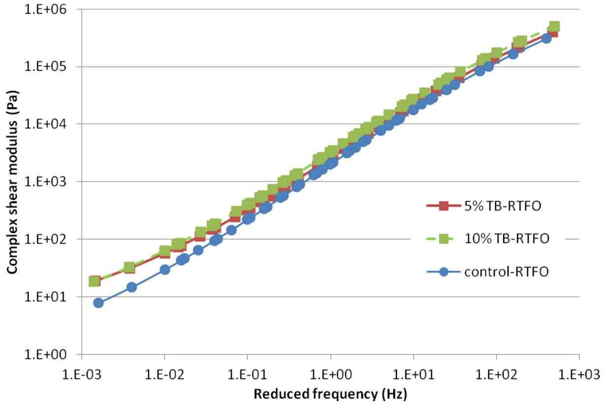
**Figure 4-12:  $G^*$  master curve plot for control binder, 5% and 10% TB modified asphalt binders after RTFO aging**
