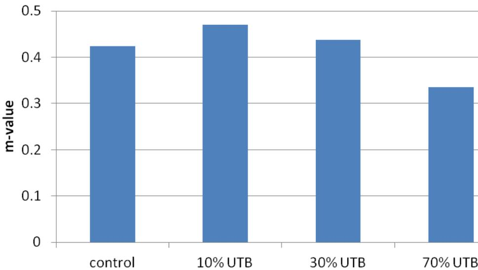
**Figure 5-17: M-value of control binder, 10%, 30% and 70% UTB bioasphalt at 60s in BBR test**
