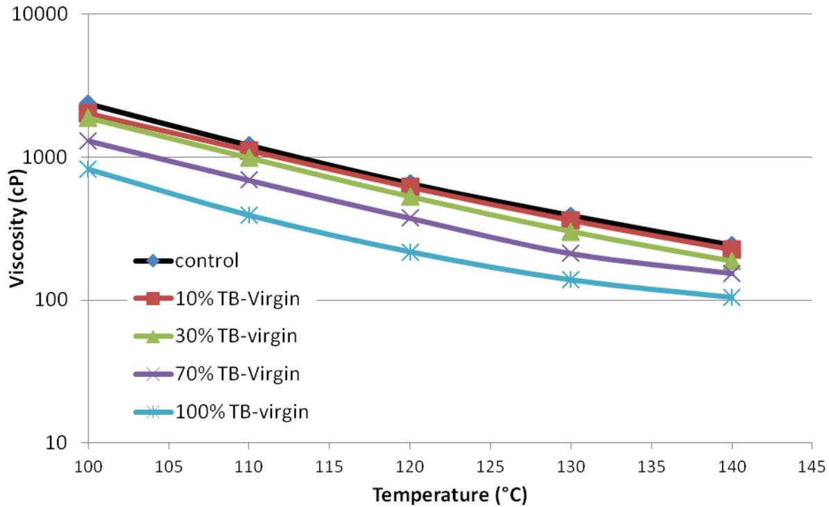
**Figure 5-2: RV test results for control asphalt binder, 10%, 30%, 70% and 100% bioasphalt binders**
