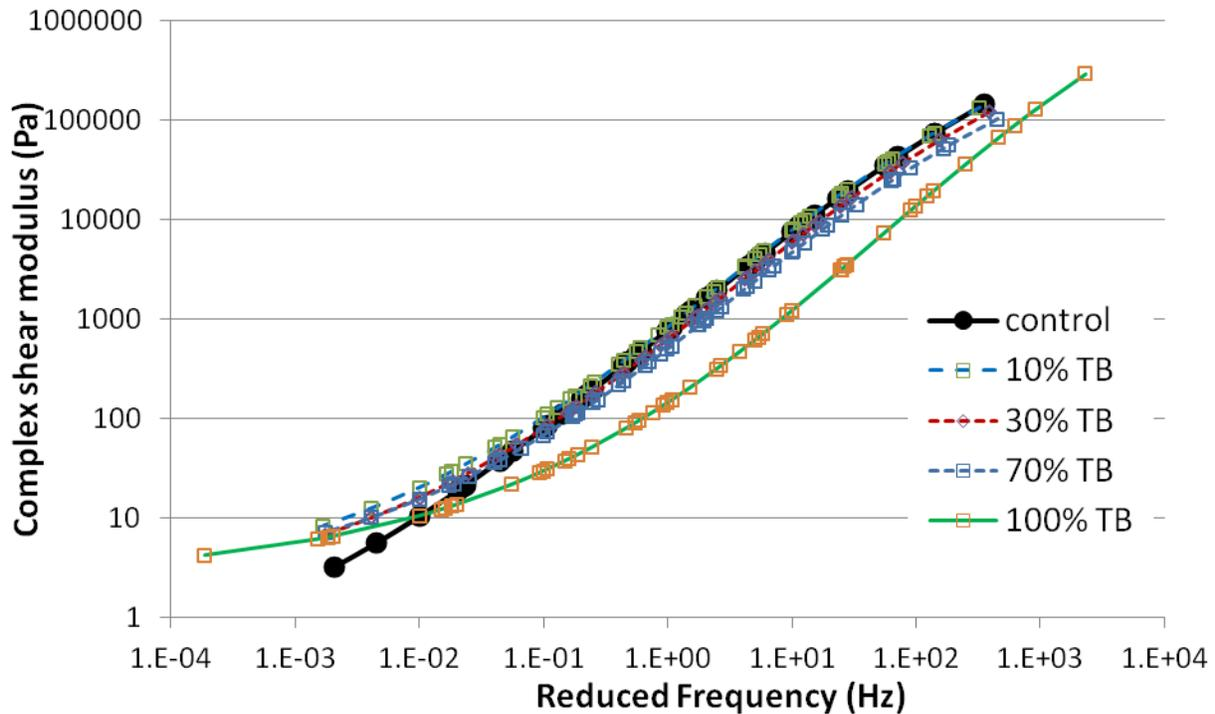
**Figure 5-9: Master curve plot for control binder, 10%, 30% and 70% TB bioasphalt binders in the temperature range of 40°C to 70°C.**
