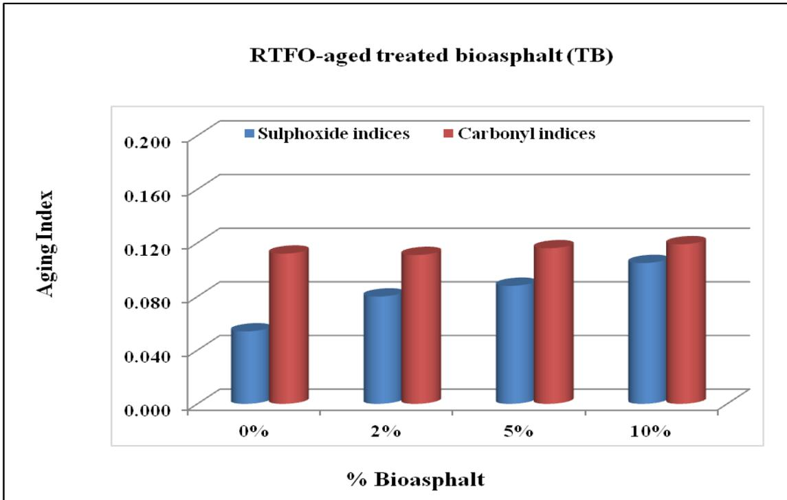
**Figure 3-8: Bar chart of aging indices for RTFO-aged control and treated bioasphalt**
