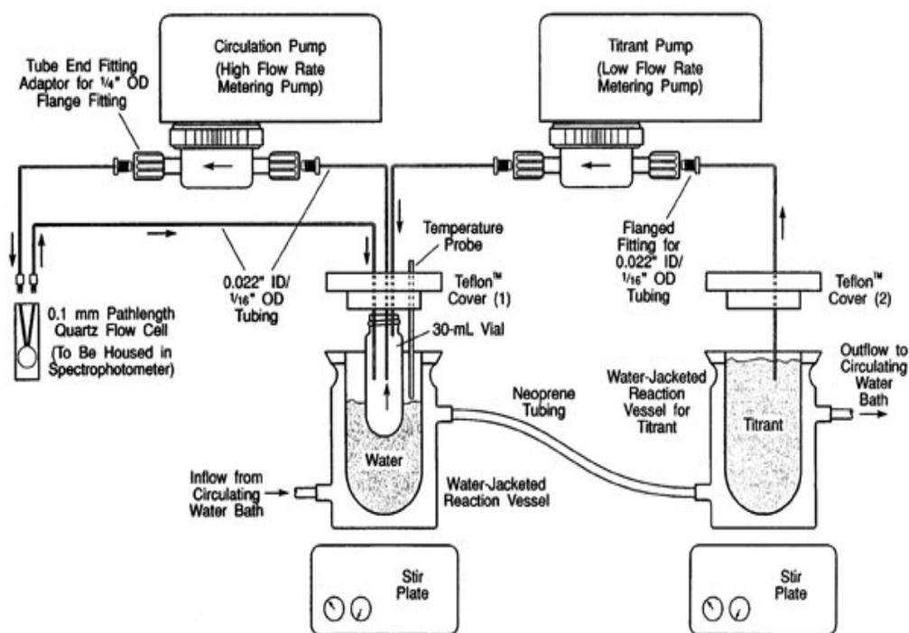
**Figure 3-1: A schematic of the Automated Flocculation Titrimetry (AFT) (Koehler 2011)**
