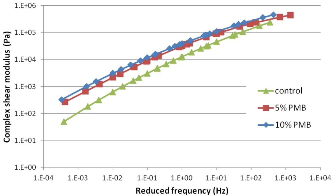
**Figure 4-18:  $G^*$  master curve plot for control binder and 5% and 10% PMB modified asphalt binders after PAV aging**
