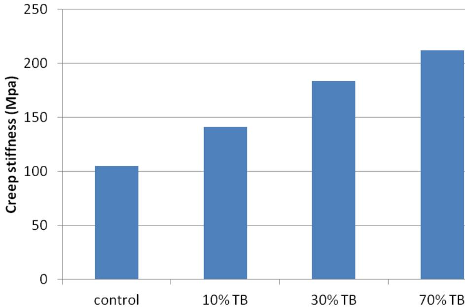
**Figure 5-18: Creep stiffness of control binder, 10%, 30% and 70% TB bioasphalt at 60s during BBR test**
