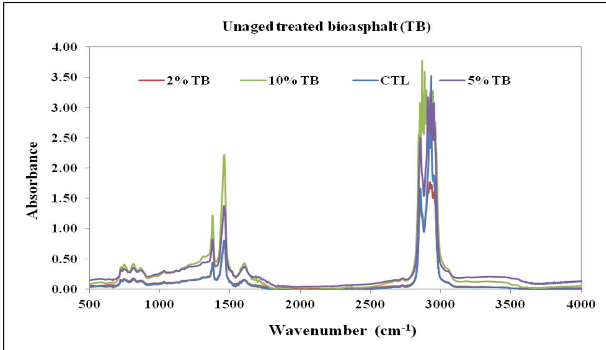
**Figure 3-4: FTIR spectra for control and treated bio oil modified PG 58-28 asphalt binder at unaged condition**
