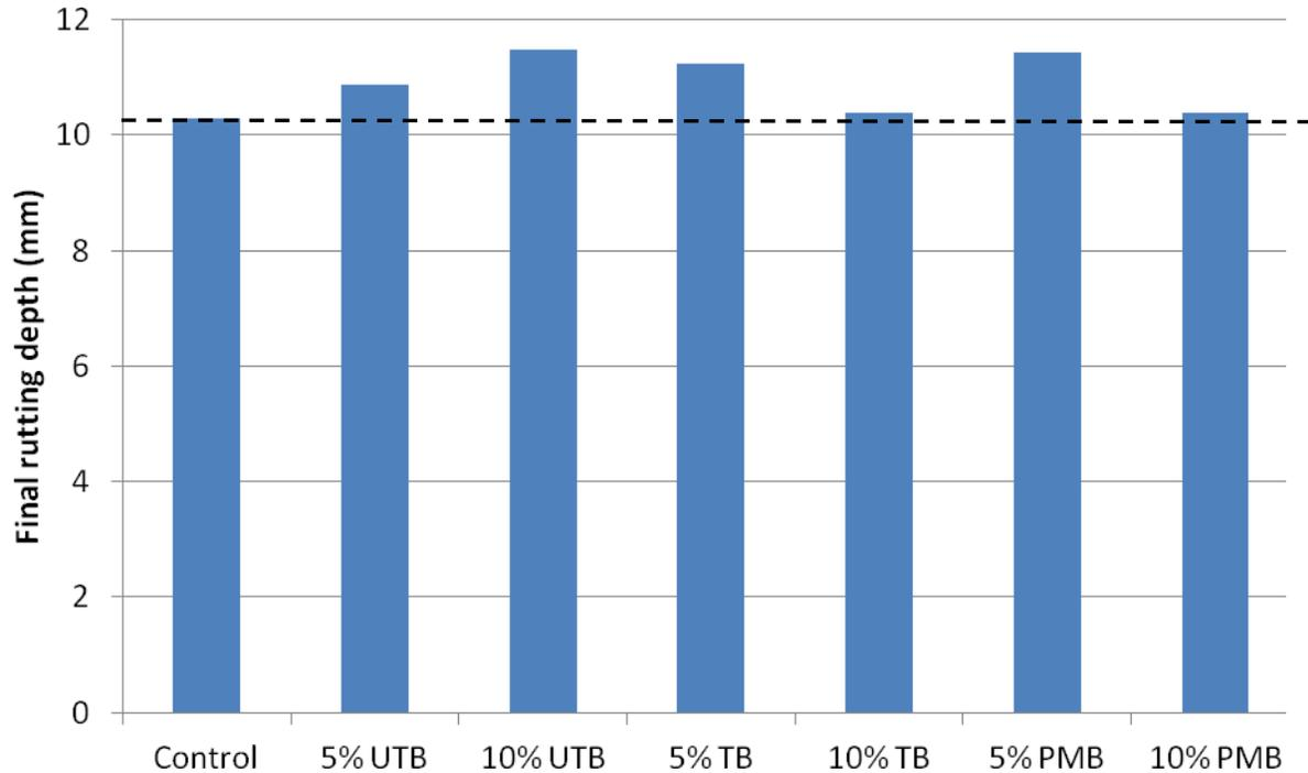
**Figure 6-7: The final rutting depth of control HMA mixture and bio oil modified HMA mixtures at 58°C**
