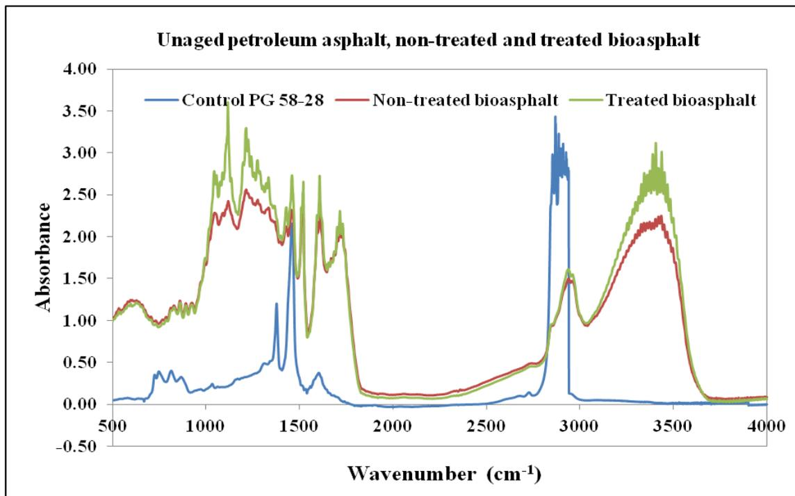
**Figure 3-2: FTIR spectra for pure petroleum asphalt (PG 58-28), untreated and treated bioasphalt at their unaged condition**
