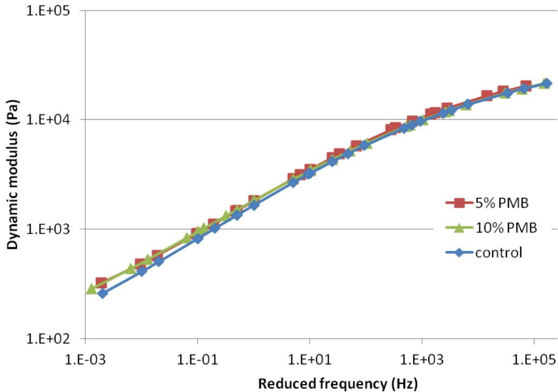
**Figure 6-4: Dynamic modulus master curve plot for control asphalt mixture, 5% and 10% PMB modified asphalt mixture**
