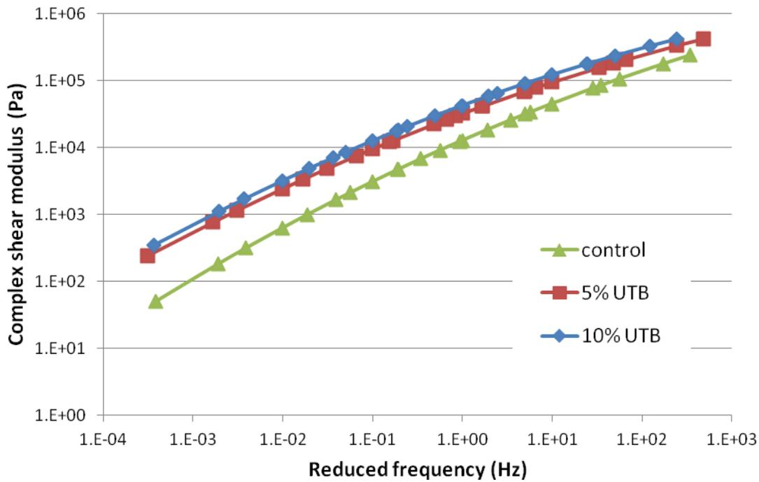
**Figure 4-16:  $G^*$  master curve plot for control binder and 5% and 10% UTB modified asphalt binders after PAV aging**
