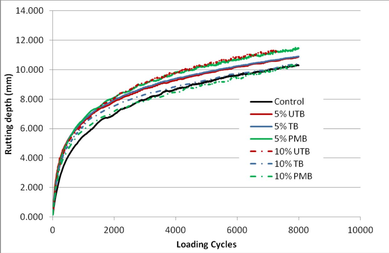
Figure 6-6: The APA test results for control HMA mixture and bio oil modified HMA mixture at 58°C
