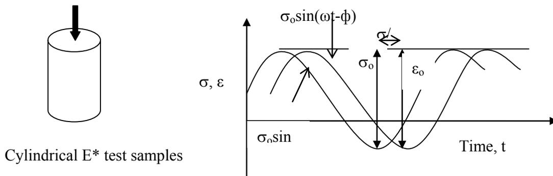
**Figure 6-1: Haversine loading pattern for the dynamic modulus test**
