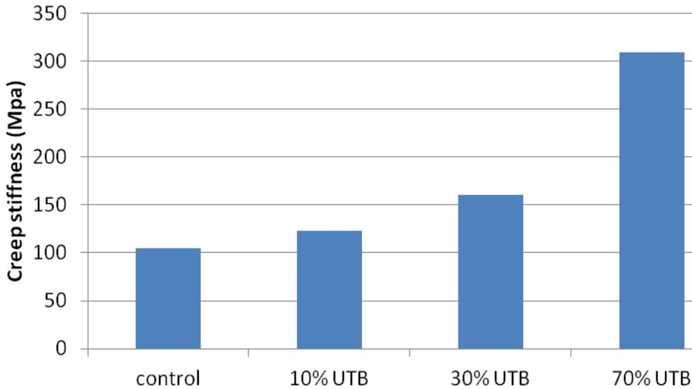
**Figure 5-16: Creep stiffness of control binder, 10%, 30% and 70% UTB bioasphalt at 60s during BBR test**
