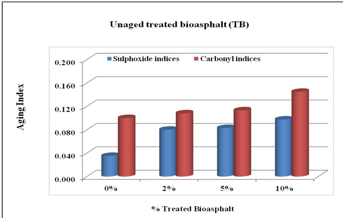
**Figure 3-6: Bar chart of aging indices for unaged control and TB modified asphalt binders**
