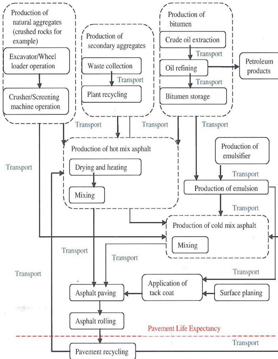
**Figure 7-2: Typical unit processes in asphalt pavement construction works**
