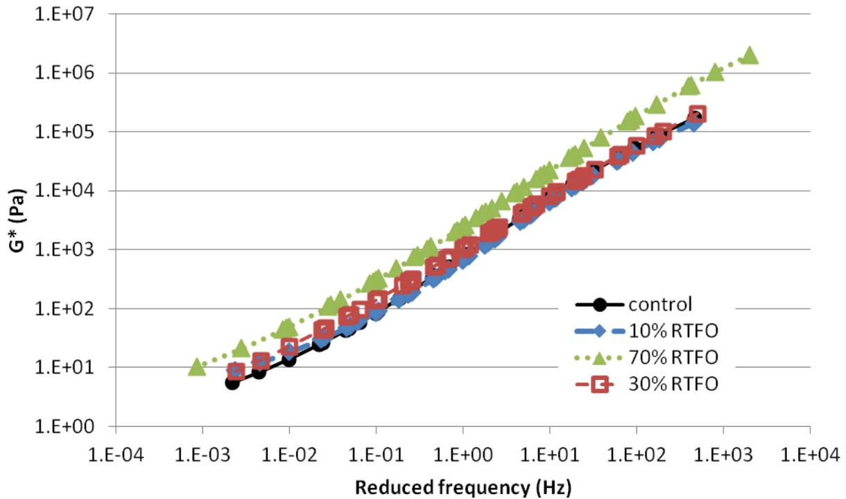
**Figure 5-11: Master curve plot for control binder, 10%, 30% and 70% UTB blended asphalt binders in the temperature range of 40°C to 70°C after RTFO aging**
