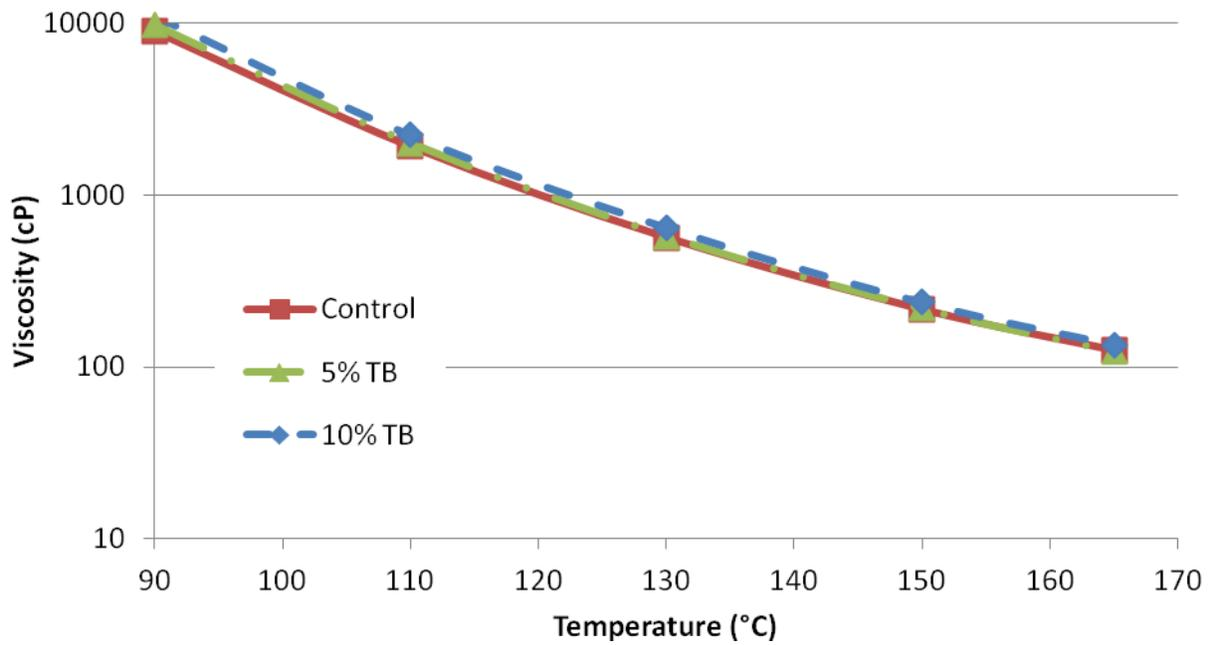
**Figure 4-5: RV test results of control binder, 5%, and 10% UTB modified binders, after RTFO aging**
