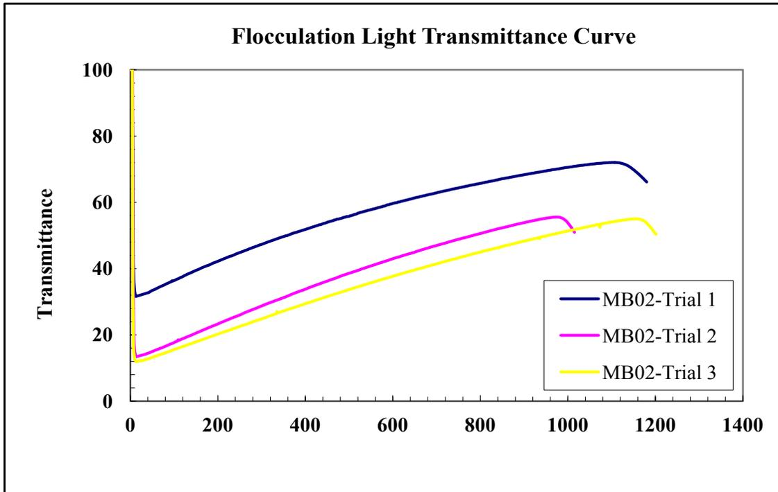
Figure 3-12: Titration time against light transmittance for control PG 58-28 binder (0% bioasphalt)
