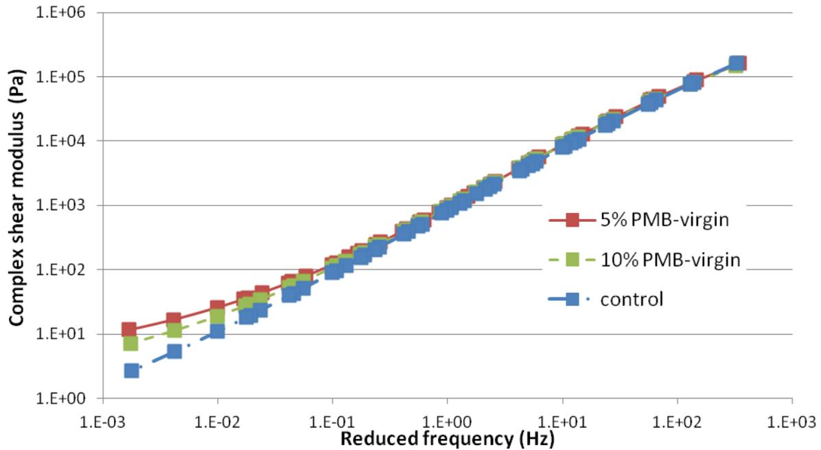
**Figure 4-10:  $G^*$  master curve for control binder, 5% and 10% PMB modified asphalt binders before RTFO aging**
