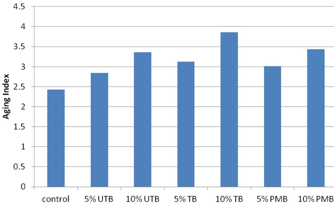
**Figure 4-14: Aging Indexes of control binder and bio oil modified asphalt binders in low temperature ranges after RTFO aging**
