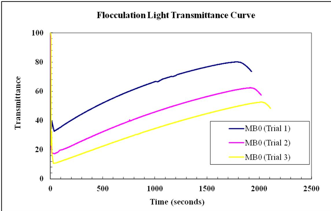
Figure 3-11: Titration time against light transmittance for control PG 58-28 binder (0% bioasphalt)
