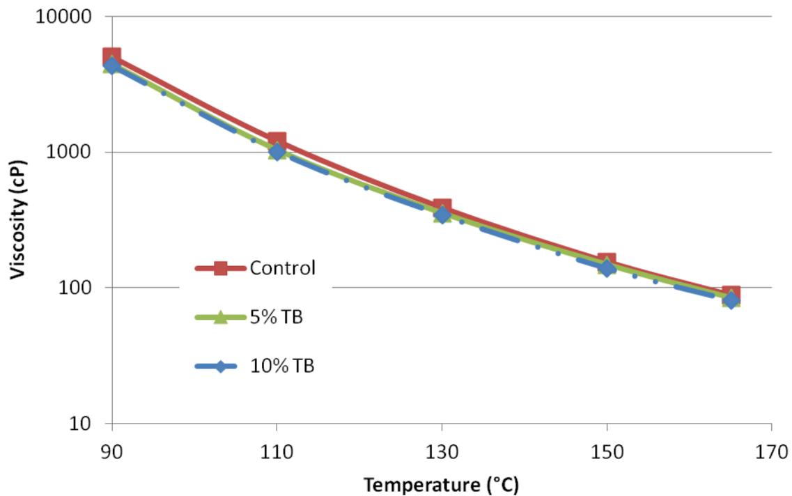
**Figure 4-3: RV test results for control binder, 5%, 10% and 100% PMB modified asphalt binders before RTFO aging**
