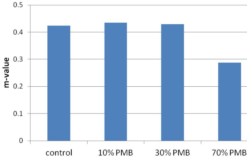
**Figure 5-21: M-value of control binder, 10%, 30% and 70% PMB bioasphalt at 60s in BBR test**
