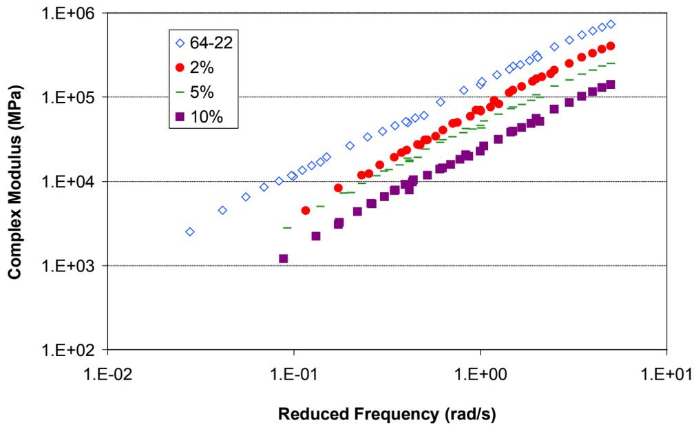
Figure 1-4: Effect of swine waste binder on petroleum-based asphalt (Fini 2010)
