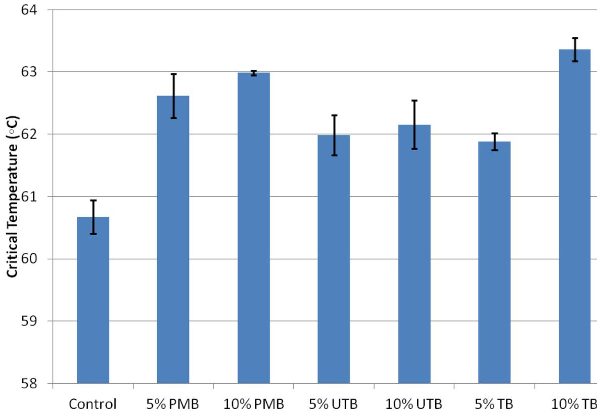
**Figure 4-15: Critical high temperatures for control asphalt binder and bio oil modified asphalt binders for rutting consideration**
