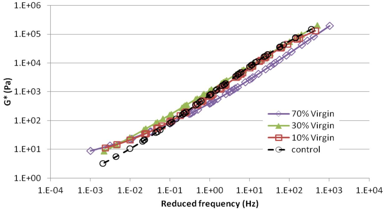
**Figure 5-7: Master curve plot for the virgin control binder, 10%, 30% and 70% UTB blended asphalt binders in temperature range 40°C to 70°C**
