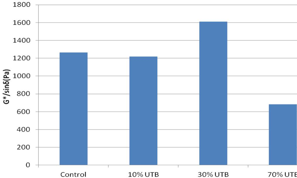
**Figure 5-8:  $G^*/\sin\delta$  values of control binder, 10%, 30% and 70% UTB bioasphalt at 58°C and 1.59Hz**
