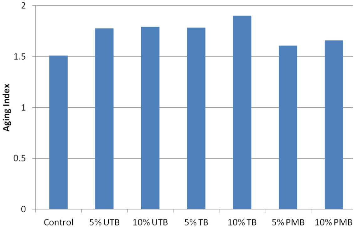
**Figure 4-7: Average aging index of control binder and bio oil modified asphalt binders at temperature 90°C, 110°C, 130°C, 150°C and 165°C from RV test**
