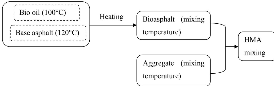
**Figure 8-1: Flow chart for the HMA mixing**
