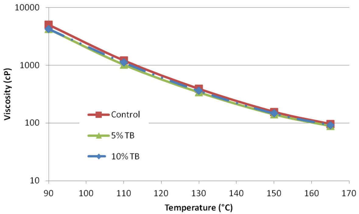
**Figure 4-2: RV test results for control binder, 5%, 10% and 100% TB modified asphalt binders before RTFO aging**
