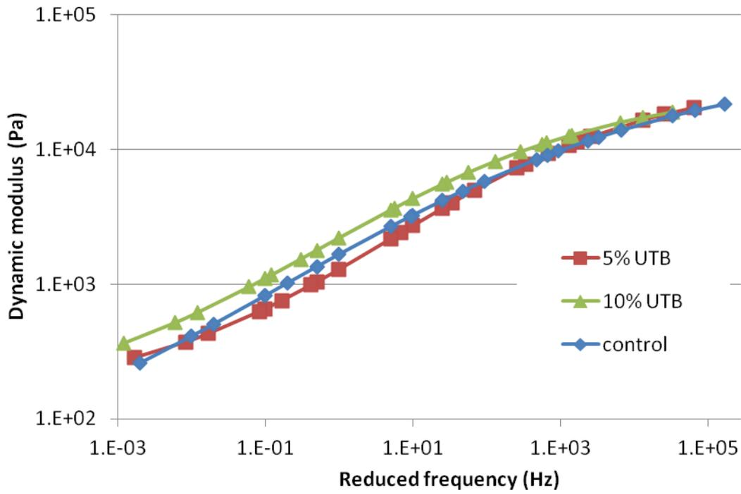
**Figure 6-2: Dynamic modulus master curve plot for control asphalt mixture, 5% and 10% UTB modified asphalt mixture**
