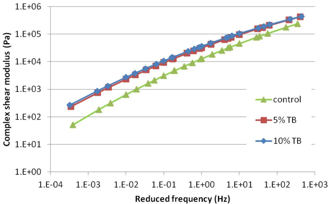
**Figure 4-17:  $G^*$  master curve plot for control binder and 5% and 10% TB modified asphalt binders after PAV aging**
