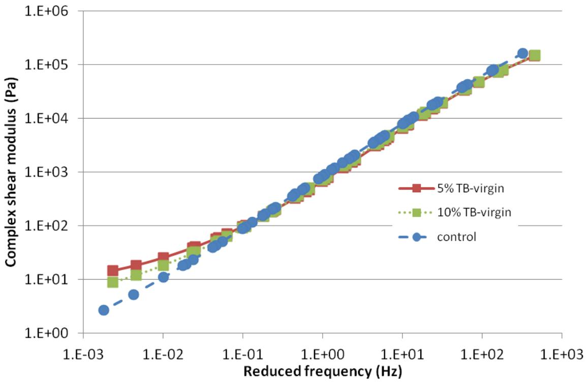
**Figure 4-9:  $G^*$  master curve for control binder, 5% and 10% TB modified asphalt binders before RTFO aging**
