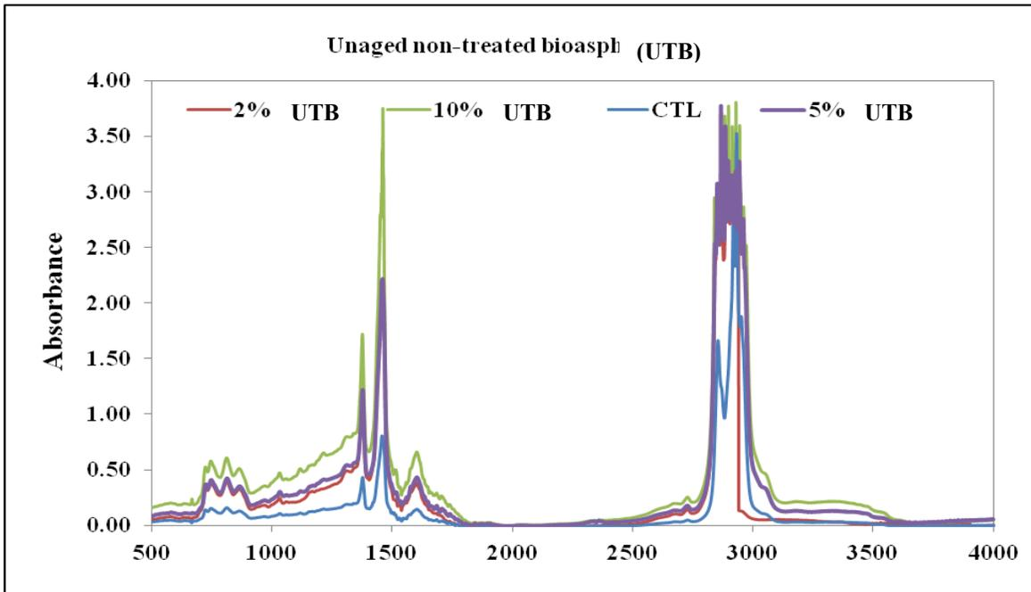
**Figure 3-3: FTIR spectra for control and untreated bio oil modified PG 58-28 asphalt binders at unaged conditions**
