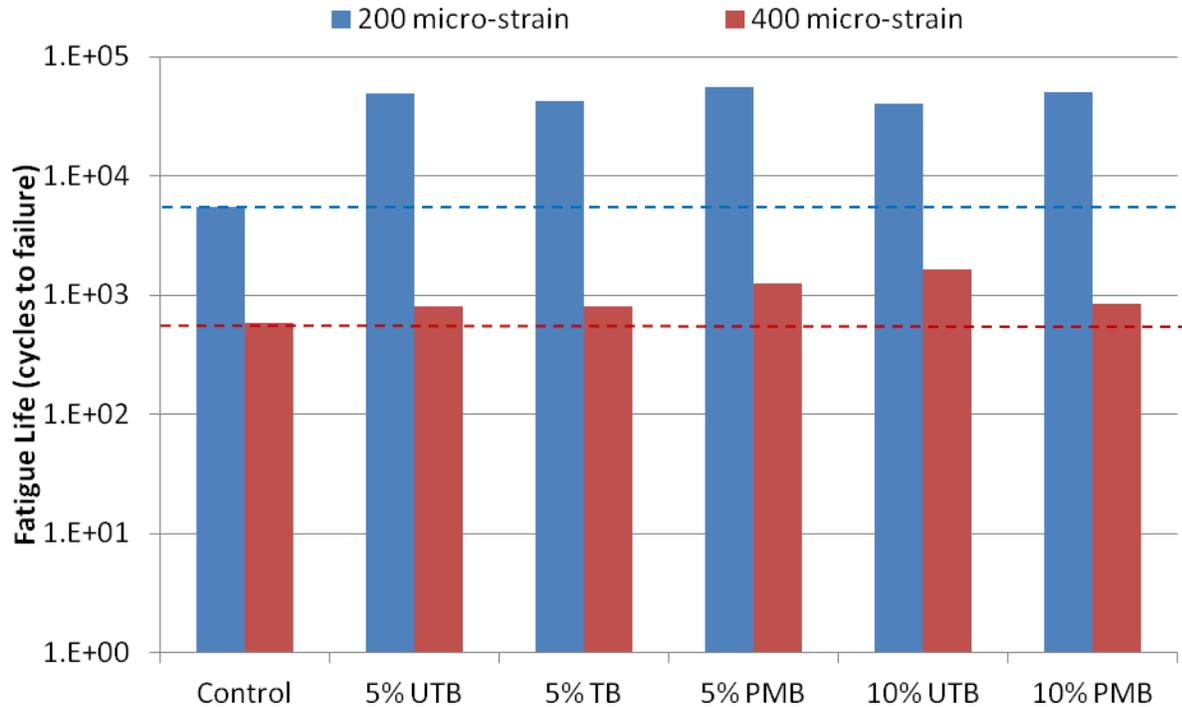
**Figure 6-11: Results of four point beam fatigue testing for control asphalt mixture, 5% UTB, 5% TB, 5% PMB, 10% UTB and 10% PMB bioasphalt mixtures**
