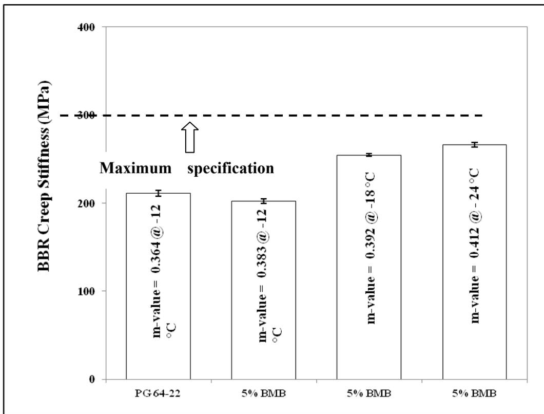
**Figure 1-6: Bar chart plots on the BBR creep stiffness behavior of samples**
