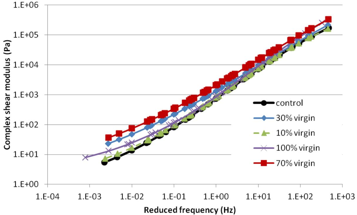
**Figure 5-10: Master curve plot for control binder, 10%, 30% and 70% PMB blended asphalt binders before RTFO aging in the temperature range of 40°C to 70°C.**
