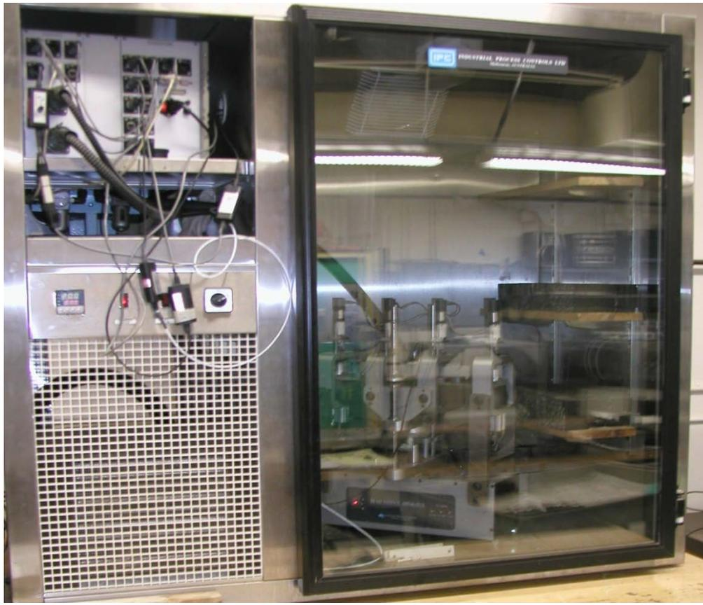
**Figure 6-10: The set-up of the four point beam fatigue test**
