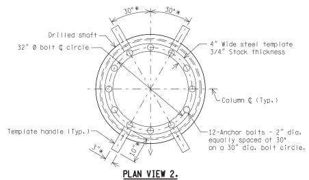
(For use with 20 ft through 30 ft cantilever arms or with 35 ft and 40 ft cantilever arms with reduced sign area (see chart on sheet 5).
