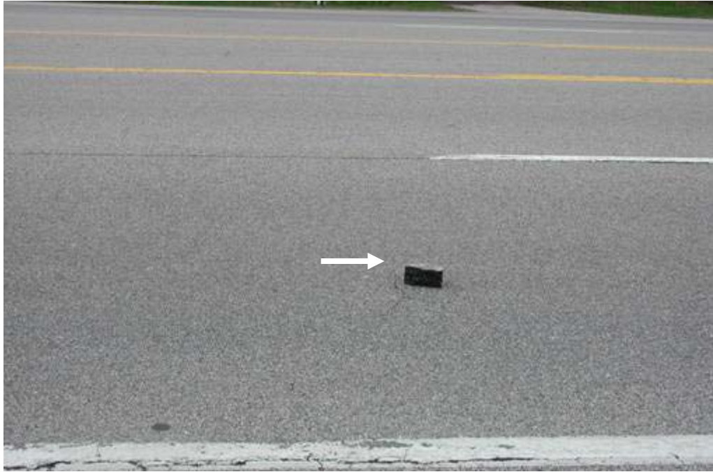
Figure 4.22 Transverse TDC located at the center of the lane (compare the size to half of a 4-in core)
