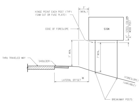
st THE LATERAL OFFSET SHALL BE 30' (MIN.), FOR MAINTENANCE PURPOSES.
