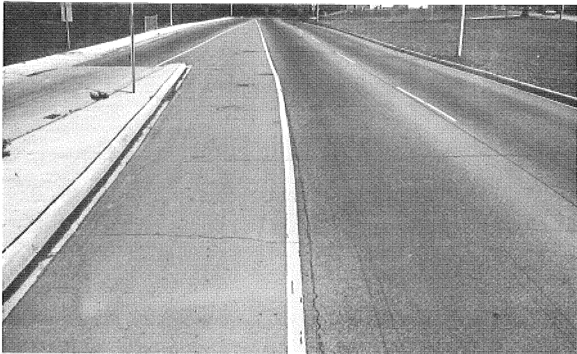
Figure 9. Markings ( (g) type) looking N on Cedar St after two years of service. Durability is still good; which is a plus for the lane lines on the most curved area in the tests (8-26-71).
