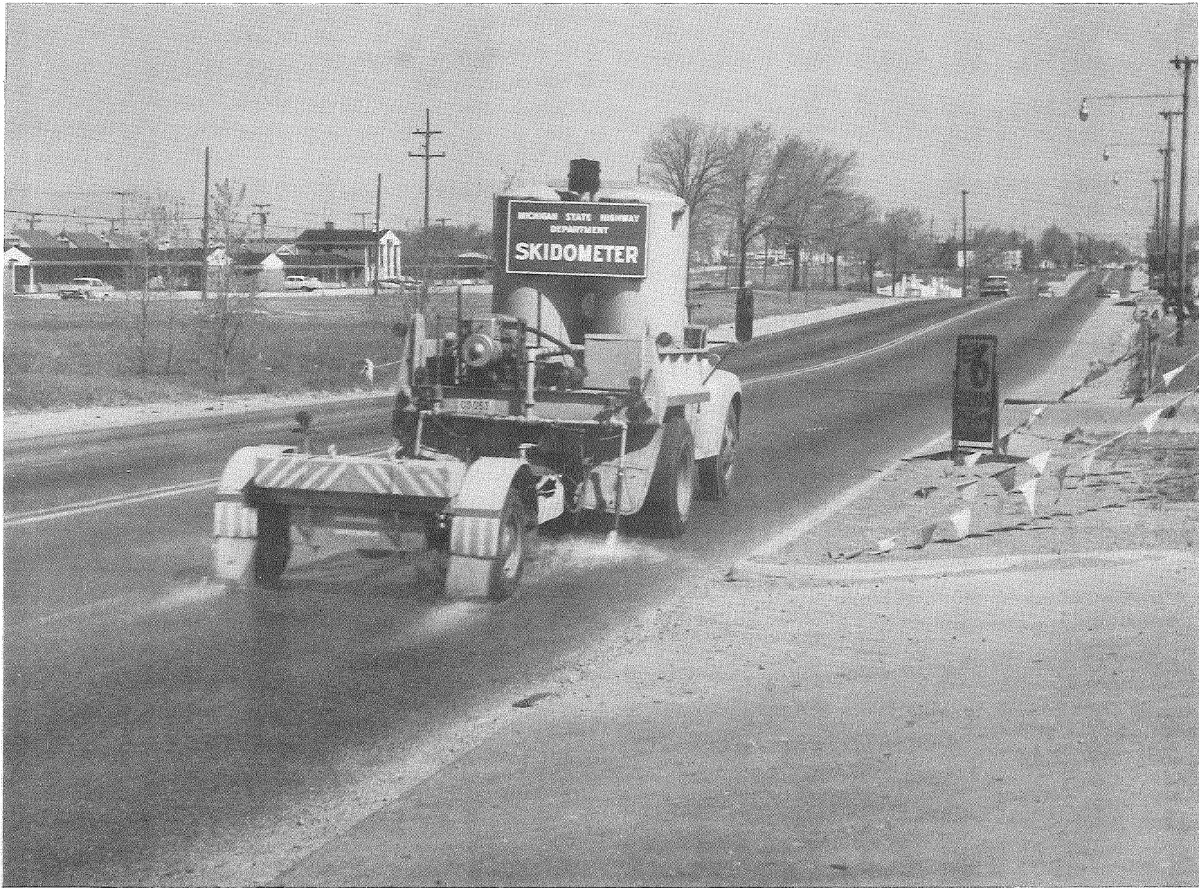
Figure 7. The MSHD Skidometer running a typical test at 40 mph on a bituminous concrete project.
