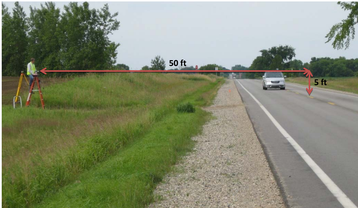
Figure 13. Example Sound Meter Setup and Test Vehicle Pass
