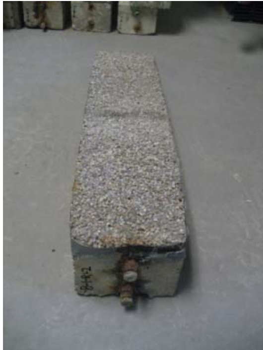
Figure 2.14 Specimen Repaired with Epoxy Overlay
