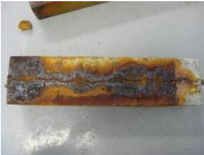
Figure 2.13 Specimen after Level 4 Corrosion
