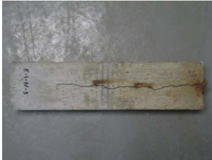
Figure 2.10 Specimen after Level 1 Corrosion
