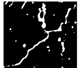
Figure B.10 B-3-N X-Ray Image and Crack after Applying Threshold
