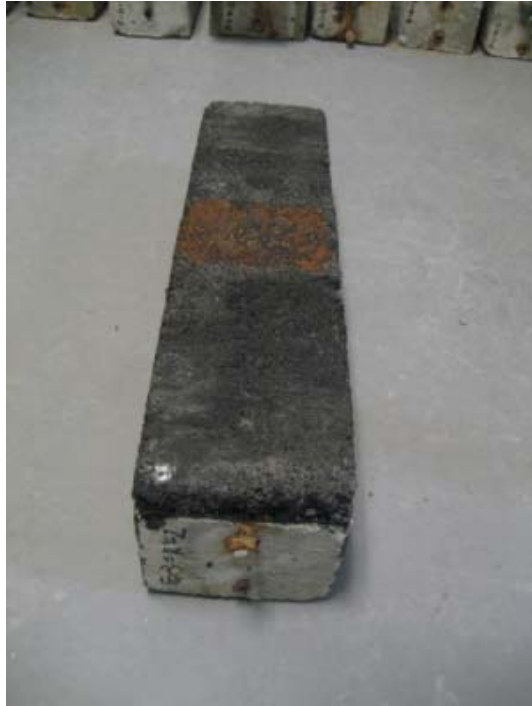
Figure 2.17 Specimen with Waterproofing and HMA Overlay
