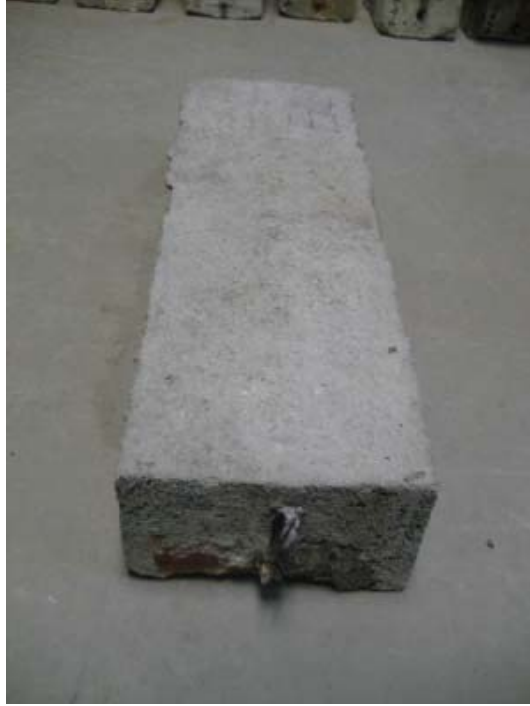
Figure 2.19 Specimen with Deep Concrete Overlay
