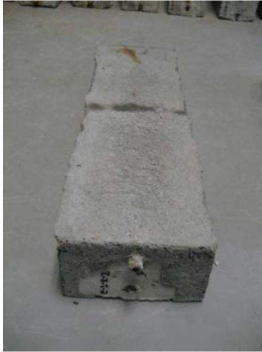
Figure 2.16 Specimen with Shallow Concrete Overlay
