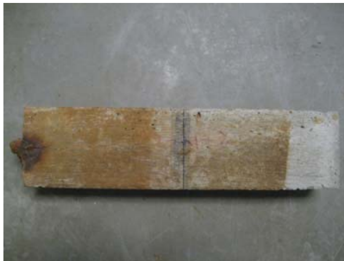
Figure 2.11 Specimen after Level 2 Corrosion
