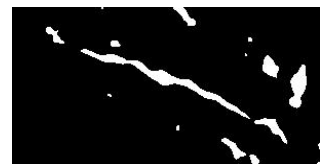
Figure B.8 B-2-R X-Ray Image and Crack after Applying Threshold
