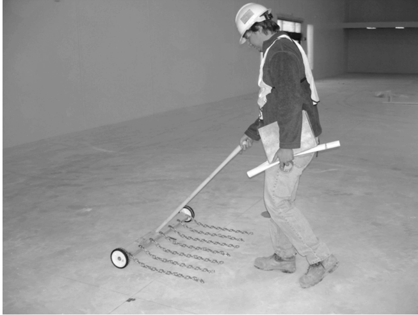
Figure 2.12 Chain Drag Test
