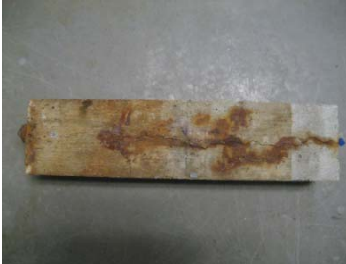
Figure 2.12 Specimen after Level 3 Corrosion
