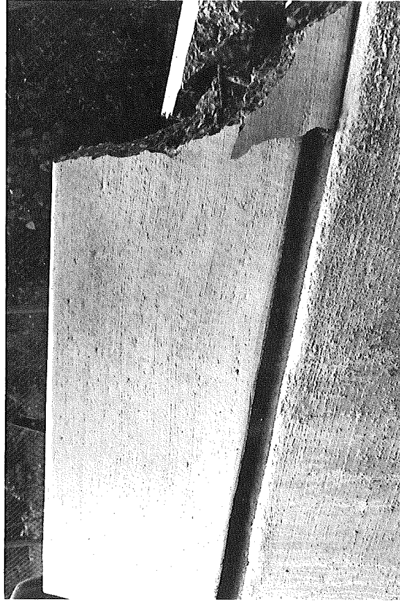
Figure 7. Results of end-loader impact on longitudinally reinforced screen.
