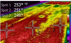
Mitigation strategies: A longitudinal joint specification could include use of a notched wedge joint (top); targeted inspection with infrared cameras during construction could help identify problematic temperature variations (bottom).
