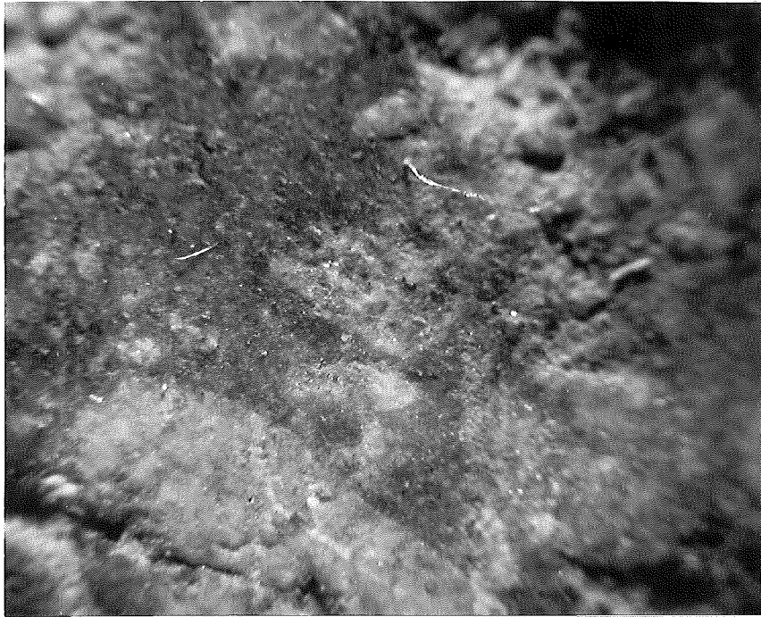
Figure 39. Texture of stone sand concrete pavement project 49-28, C2. Core 672. Unscaled surface. Magnification, 24X.
