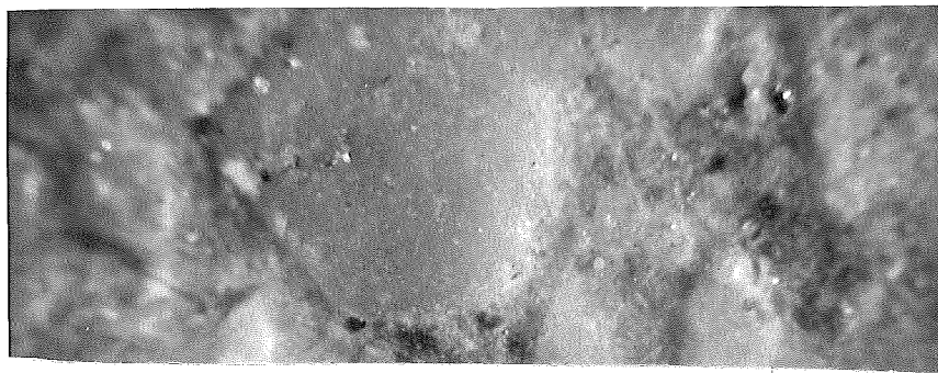
Figure 31. Texture of stone sand concrete surface. Project 75-30, C3. Note smoothness of exposed aggregate. Magnification, 24X. Core 635.
