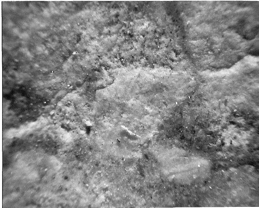
Figure 38. Texture of stone sand concrete pavement project 49-30, C9. Core 670. Unscaled surface. Magnification, 24X.
