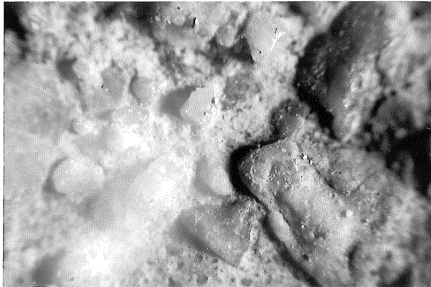
Figure 31. Texture of stone sand concrete surface. Project 75-30, C3. Note smoothness of exposed aggregate. Magnification, 24X. Core 635.
