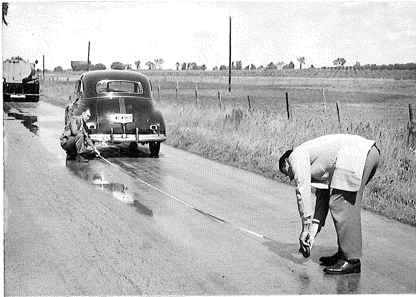
Figure 8. View showing water truck, skidding car and measurement of stopping distance.
