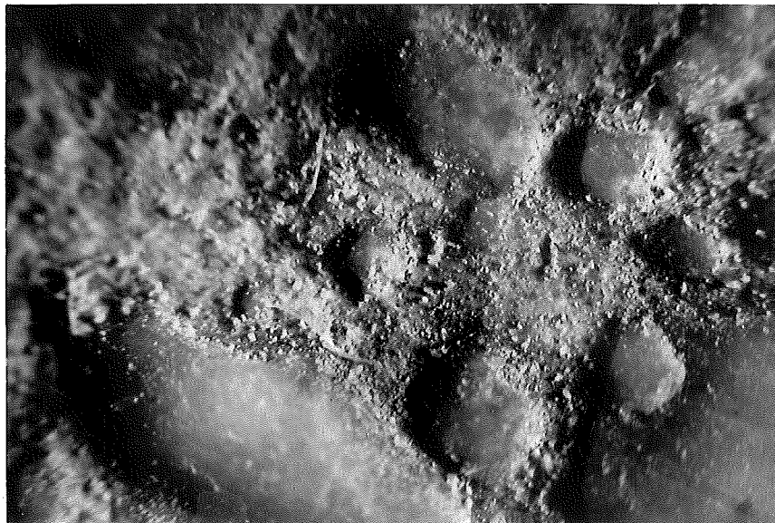
Figure 33. Texture of stone sand concrete surface. Project 75-31, C4. Core 668. Similar to Figures 31 and 32. Magnification, 24X.
