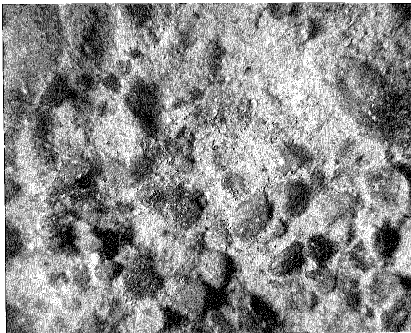
Figure 30. Texture of natural sand concrete surface. Project 75-6, C4. Core 637. Note rough, uneven surface and sand grains. Magnification, 24X.
