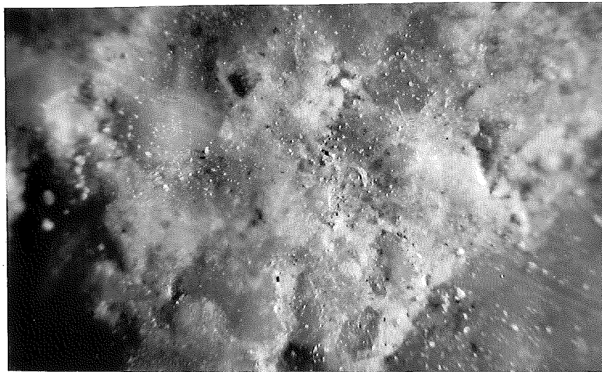
Figure 35. Texture of stone sand concrete surface project 21-29, C7. Core 630. Scaled area. Magnification, 24X.
