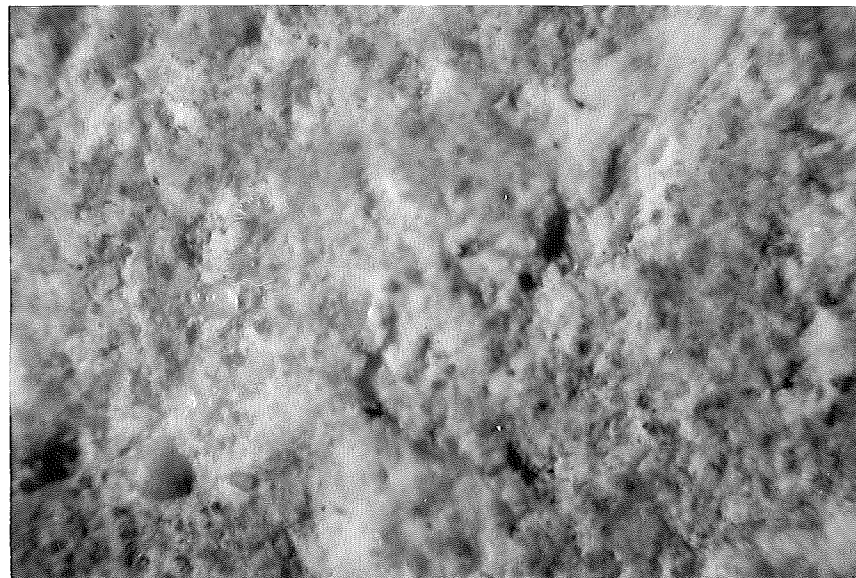
Figure 36. Texture of stone sand concrete surface, project 21-29, C7. Core 631. Unscaled area. Magnification, 24X.
