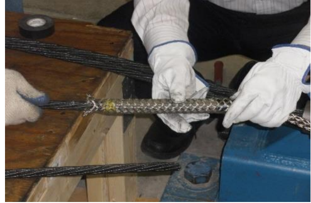
Steel braided mesh to increase friction
