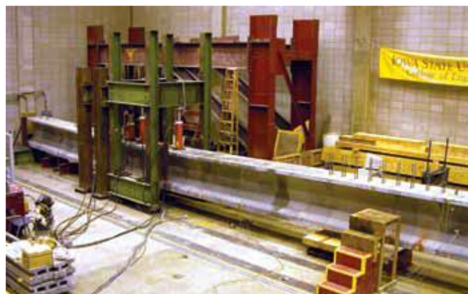
Figure 1.4-7 Flexural/shear load testing of a full-scale I girder beam (Iowa DOT 2011)
