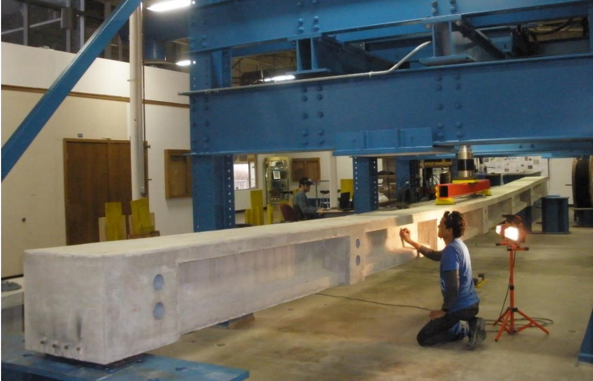
Figure 3.2-3 Crack mapping between load cycles
