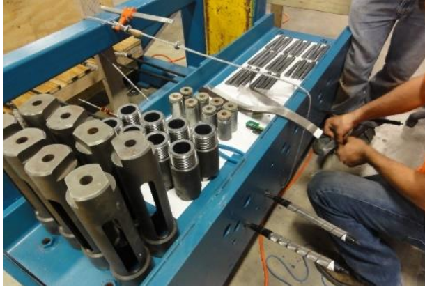
Attaching buffer material to CFCC strands
