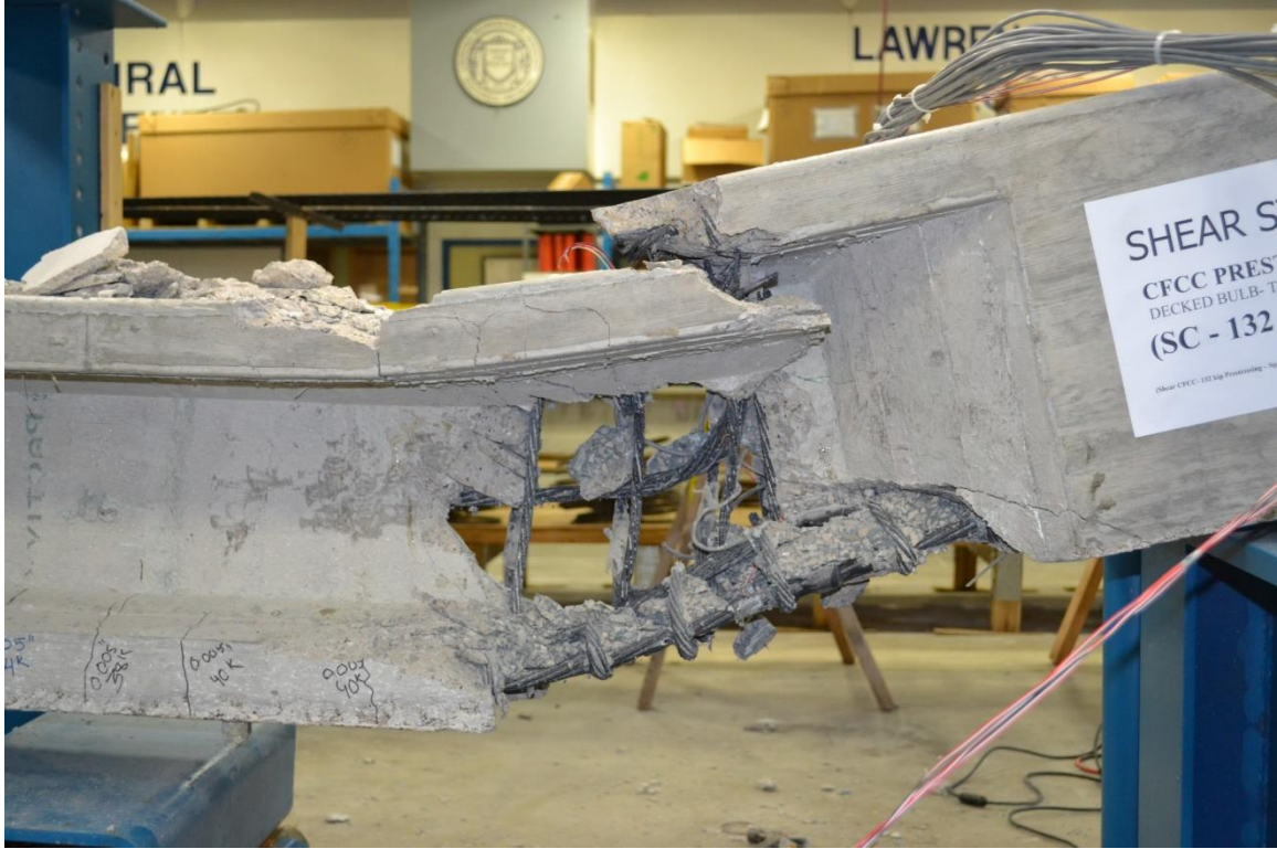
Figure 3.7-10 No rupture of CFCC stirrups was observed in Beam C-C-S-B
