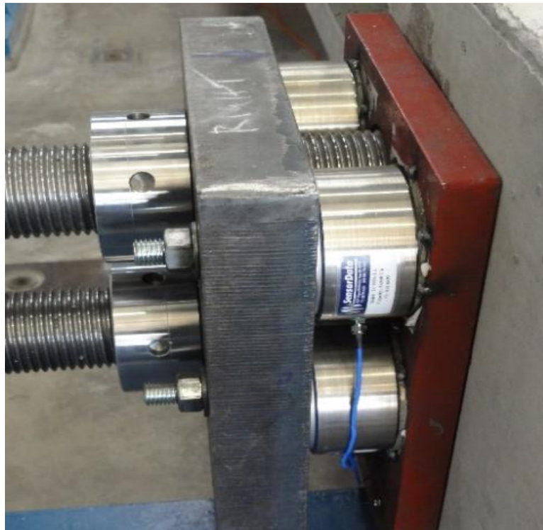
Figure 2.5-22 Load cells to monitor the transverse post-tensioning force
