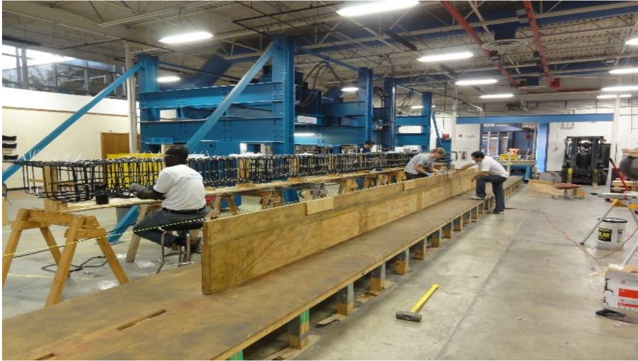
Figure 2.4-5 Wood platform decking system
