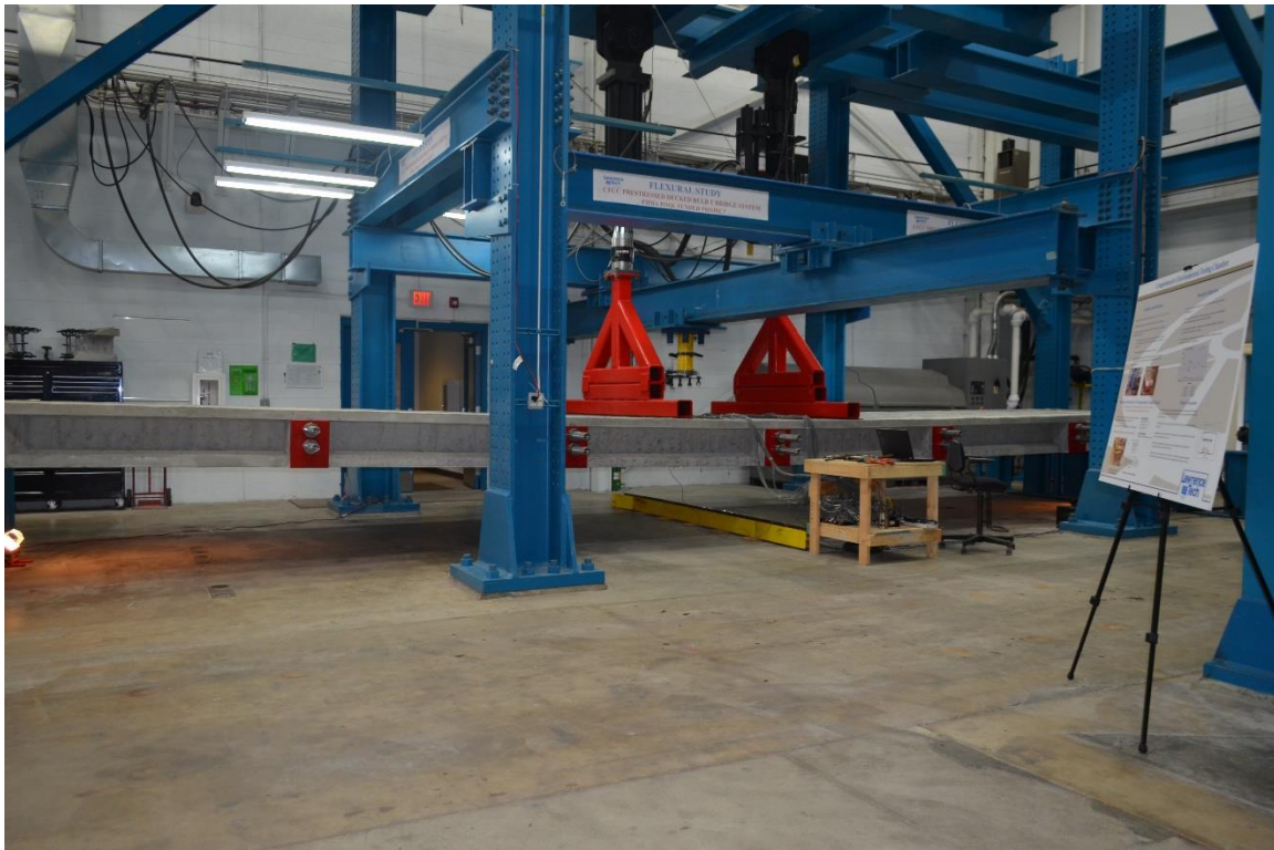
Figure 3.8-19 Load cycle test of bridge model
