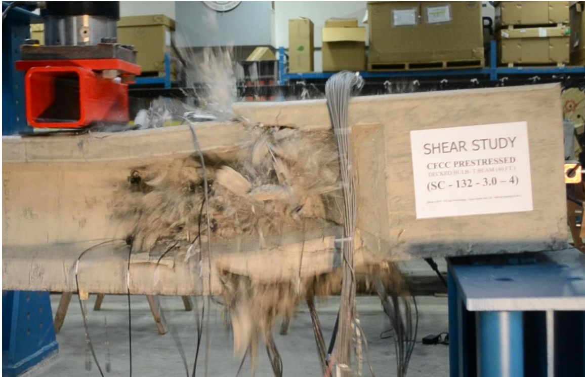
Figure 3.7-8 Explosive failure of Beam C-C-S-B
