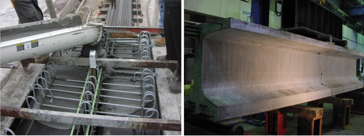
Figure 1.4-15 Building and testing UHPC bulb T beam (Ozyildirim 2011)
