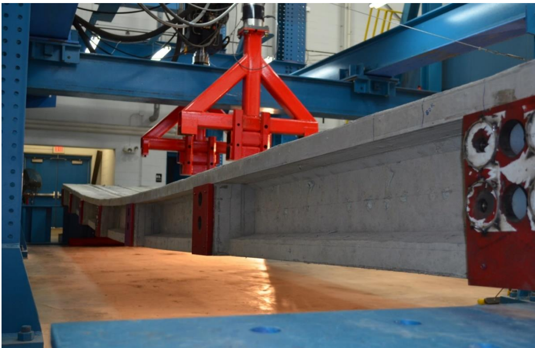
Figure 3.8-26 Bridge model at failure
