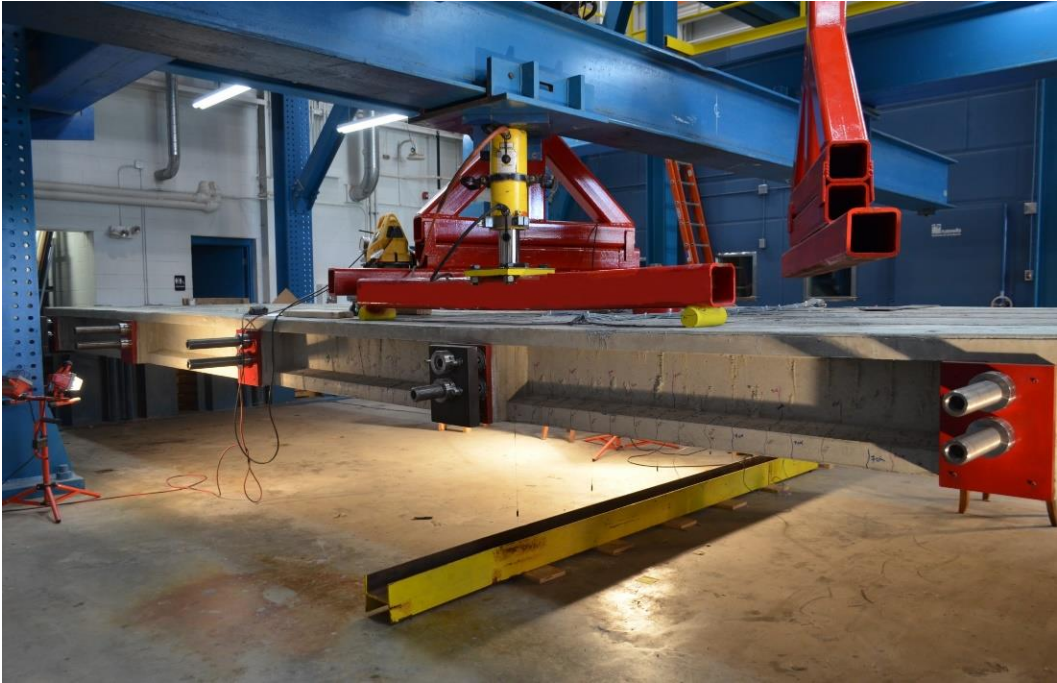
Figure 3.8-14 Shear key testing of bridge model
