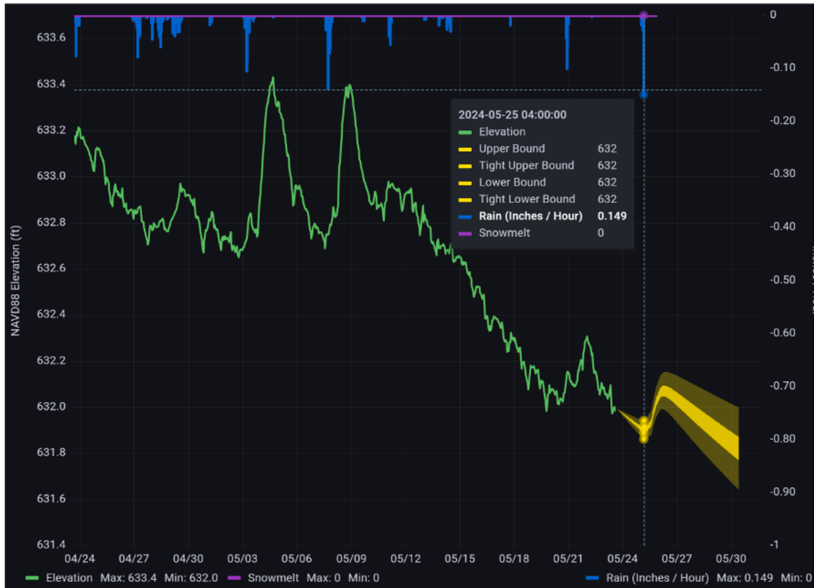
Figure 20. Sample forecasting support dashboard. Estimated snowmelt and rainfall (across all flow-distance regions) are indicated on top of the graph in purple and blue respectively. Historical water surface elevation is in green. Predictions with uncertainty estimates are provided in yellow.
