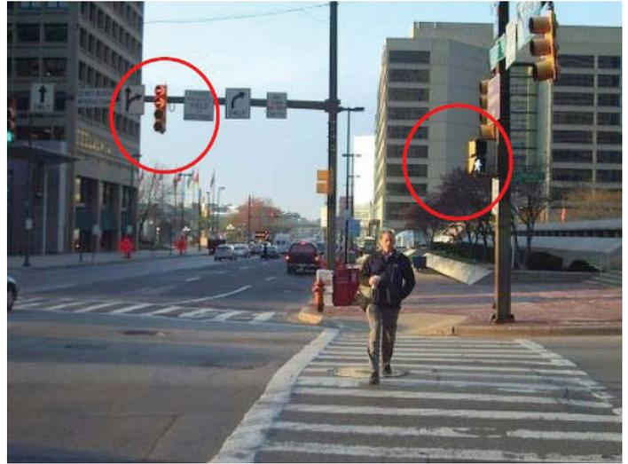
Figure 3. LPI provides head start for pedestrians (Photo Credit: *Improving Walkability at Signalized Intersections with Signal Control Strategies*)
