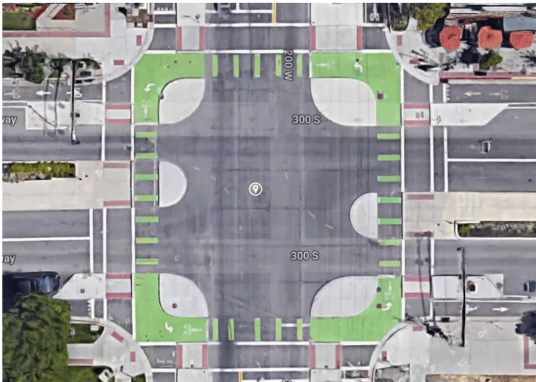
Figure 18. Protected intersection design in Salt Lake City, Utah (Photo Credit: Imagery @2018 Google)
