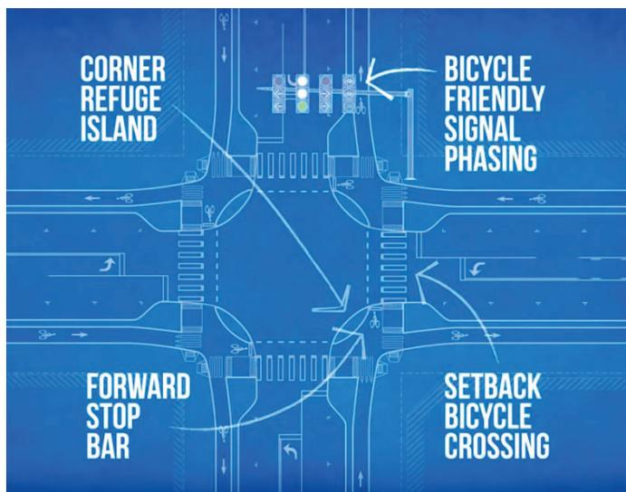
Figure 17. Design elements of protected intersections (Photo Credit: Alta Planning)
