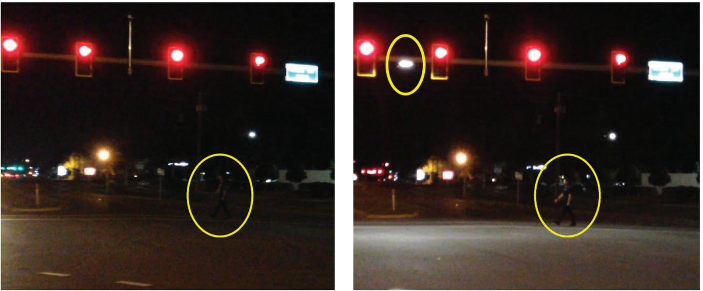
Figure 19. Before and after LED installation for pedestrian dressed in dark clothing (Photo Credit: Innovative Intersection Light Design for Pedestrian Presentation)
