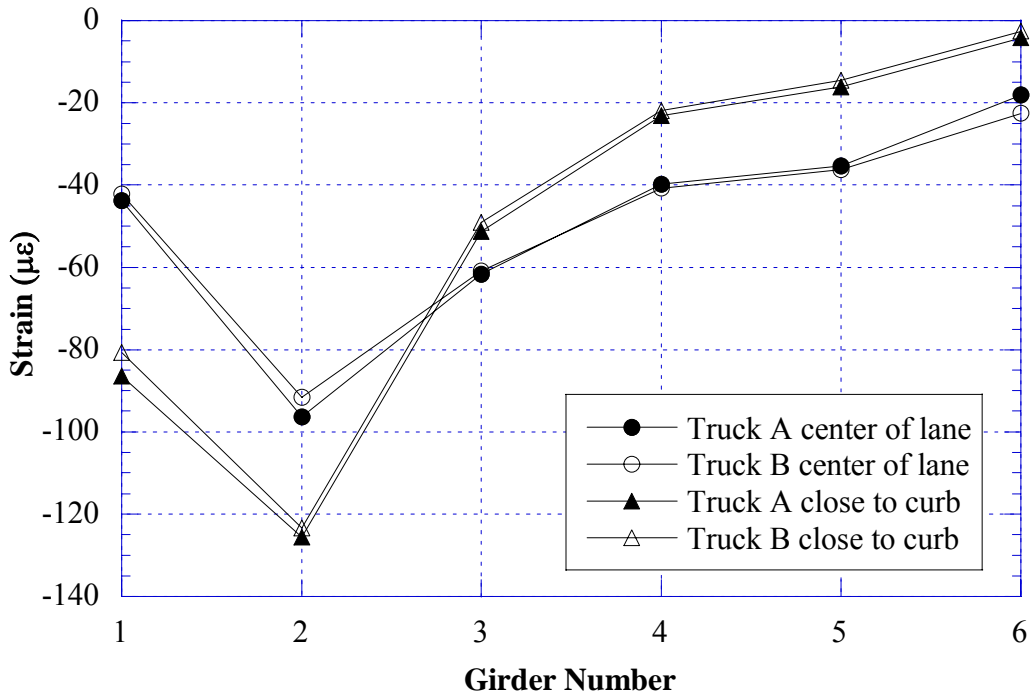
Figure 9.10 Negative Strain near Support over South Pier, East Lane Loading (S09-77023)
