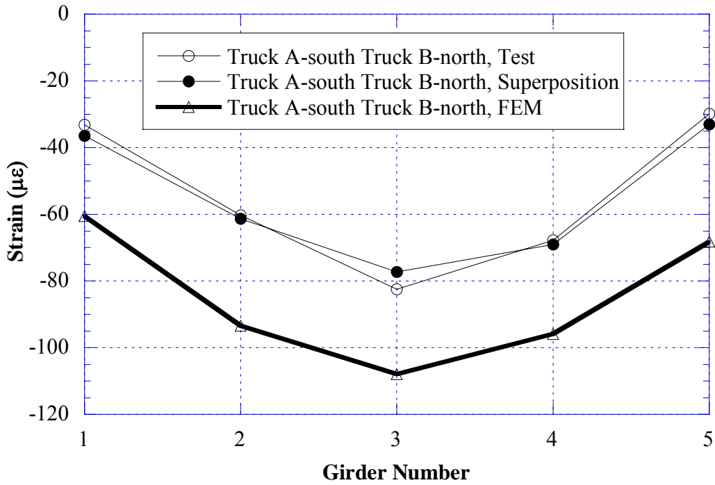
Figure 10.38 Comparison of FEM vs. Test, Negative Strain near Support over East Pier, Side-by-Side Loading (S13-59012)
