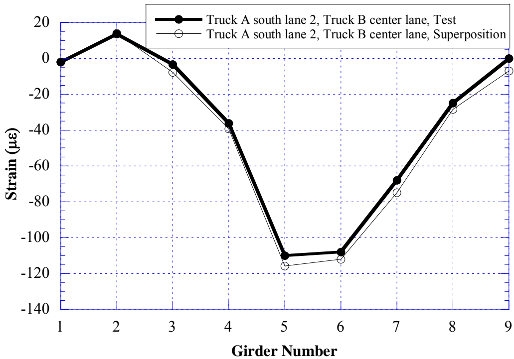
Figure 11.28 Negative Strain near Support over Center Pier, Two Truck Side-by-Side Loading, South Lane 2 and Center Lane (S12-82293)
