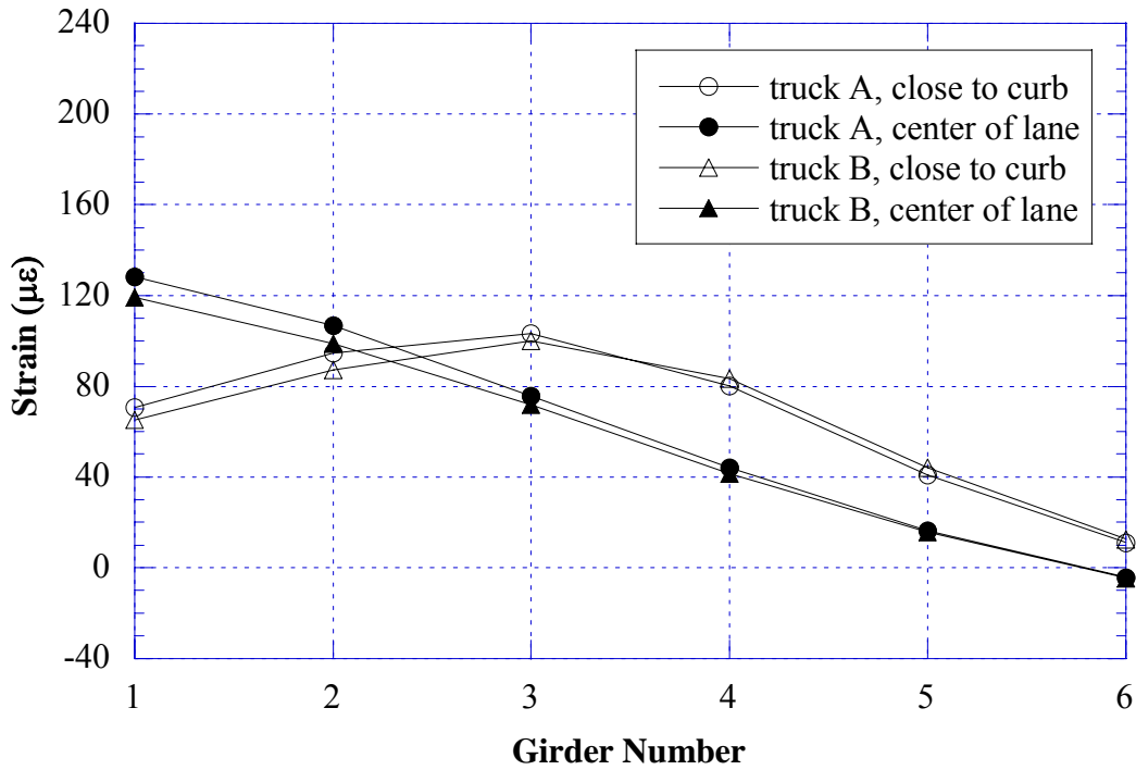
Figure 6.8 Positive Strain at Midspan of Centerspan, East Lane Loading (S08-77024)
