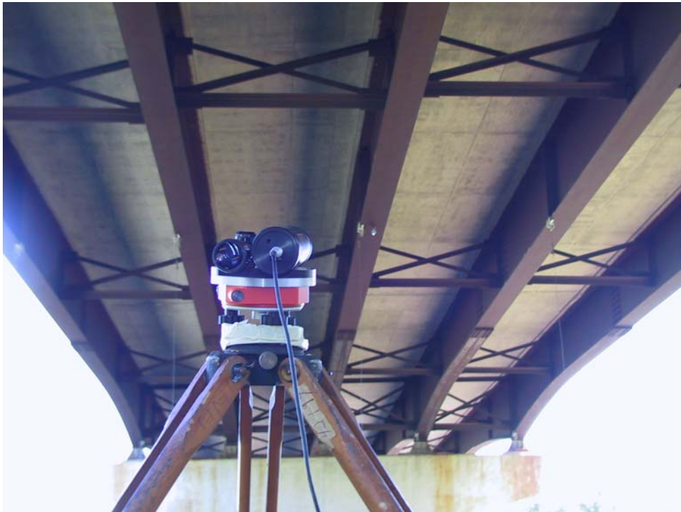
Figure 3.2 Infrared Beam Projector Manufactured by Noptel Inc. for Deflection Measurement
