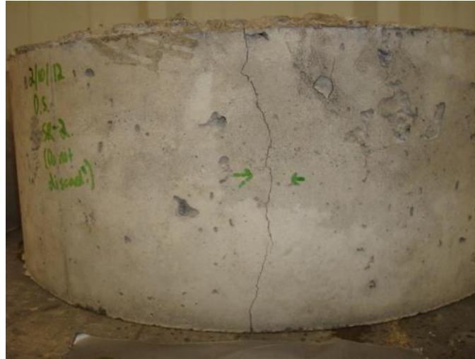
Figure 93. Ring test cracking (Ring 2)
