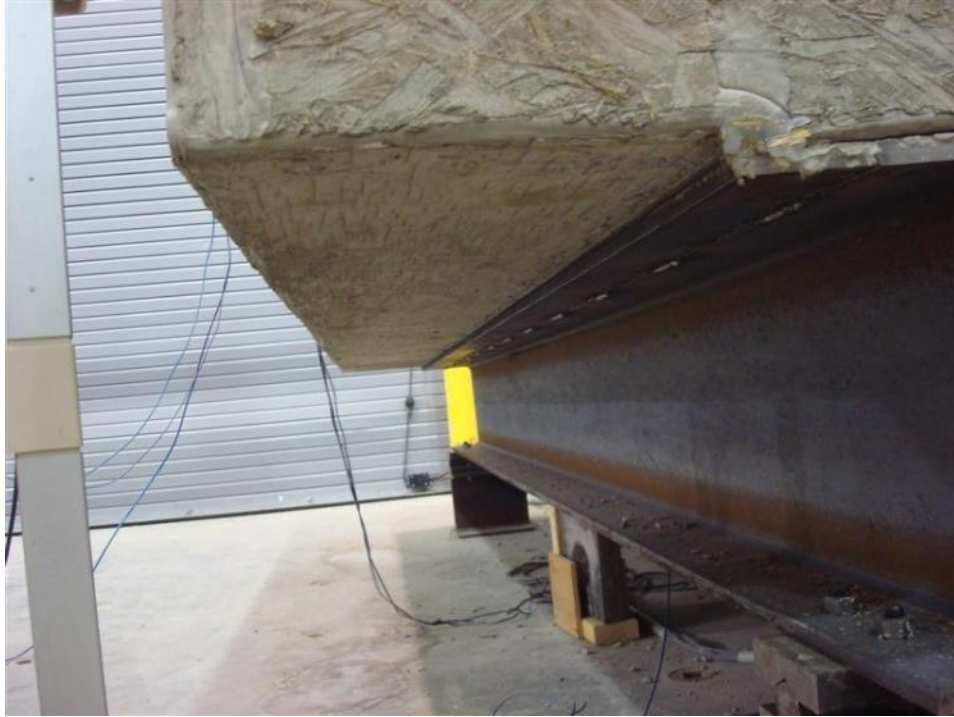
Figure 59. Completed test unit cantilever section (test unit 3)
