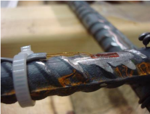
c) Lead wires adjusted so they do not touch the steel
