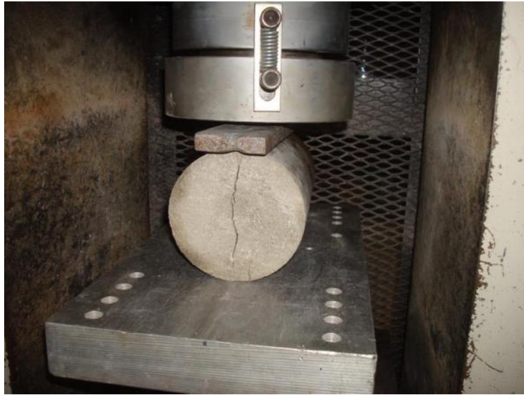
Figure 63. Concrete split tensile strength testing
