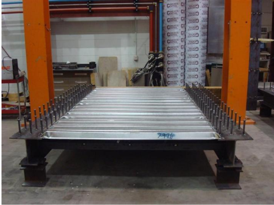
Figure 42. SIP forms front view
