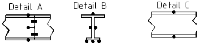
Figure 35. Steel beam strain gage locations
