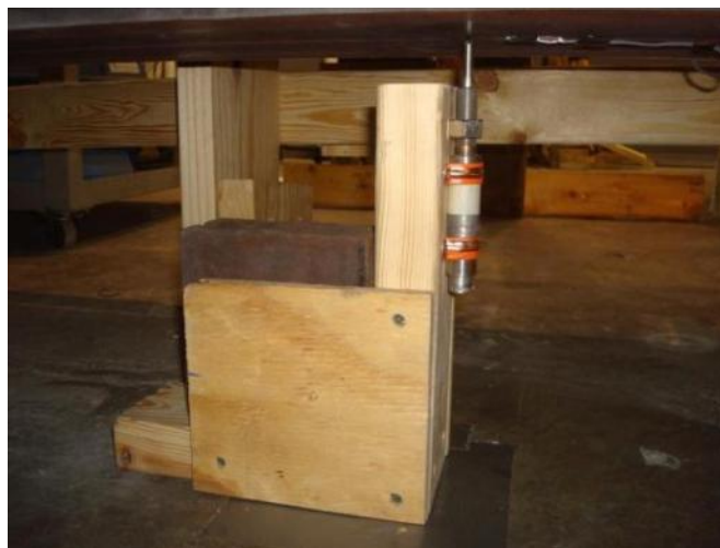
Figure 54. LVDT in place (mid-span of beam)
