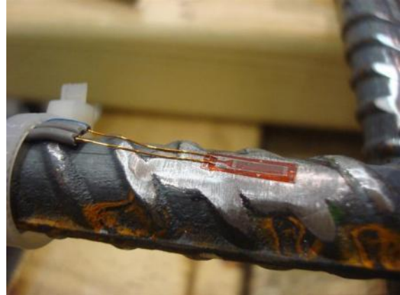
b) Strain gage attached to steel bar
