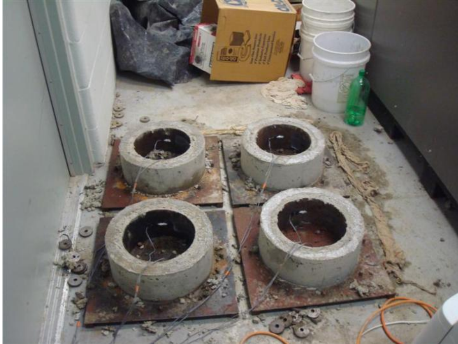
Figure 62. Overall view of shrinkage rings
