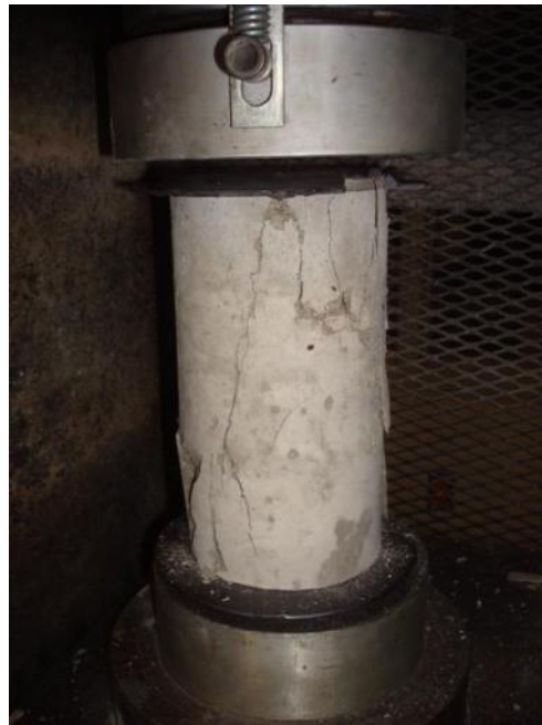
Figure 64. Concrete compressive strength testing
