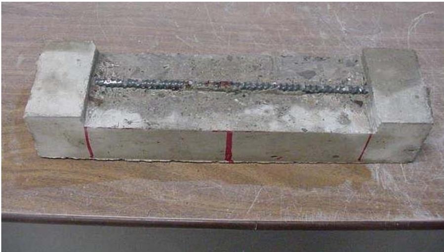
**Figure 4-32:** Specimen with expanded cavity
