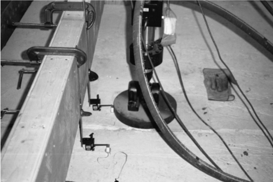
Figure 6.2 Overview of test set-up: loading plate, extensometers for measuring vertical deflections and location for measuring surface crack width is shown.
