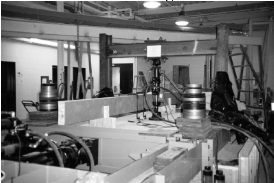
Figure 6.1 Large-scale testing frame with view of slab, horizontal and vertical actuator, reference beam, and extensometers.
