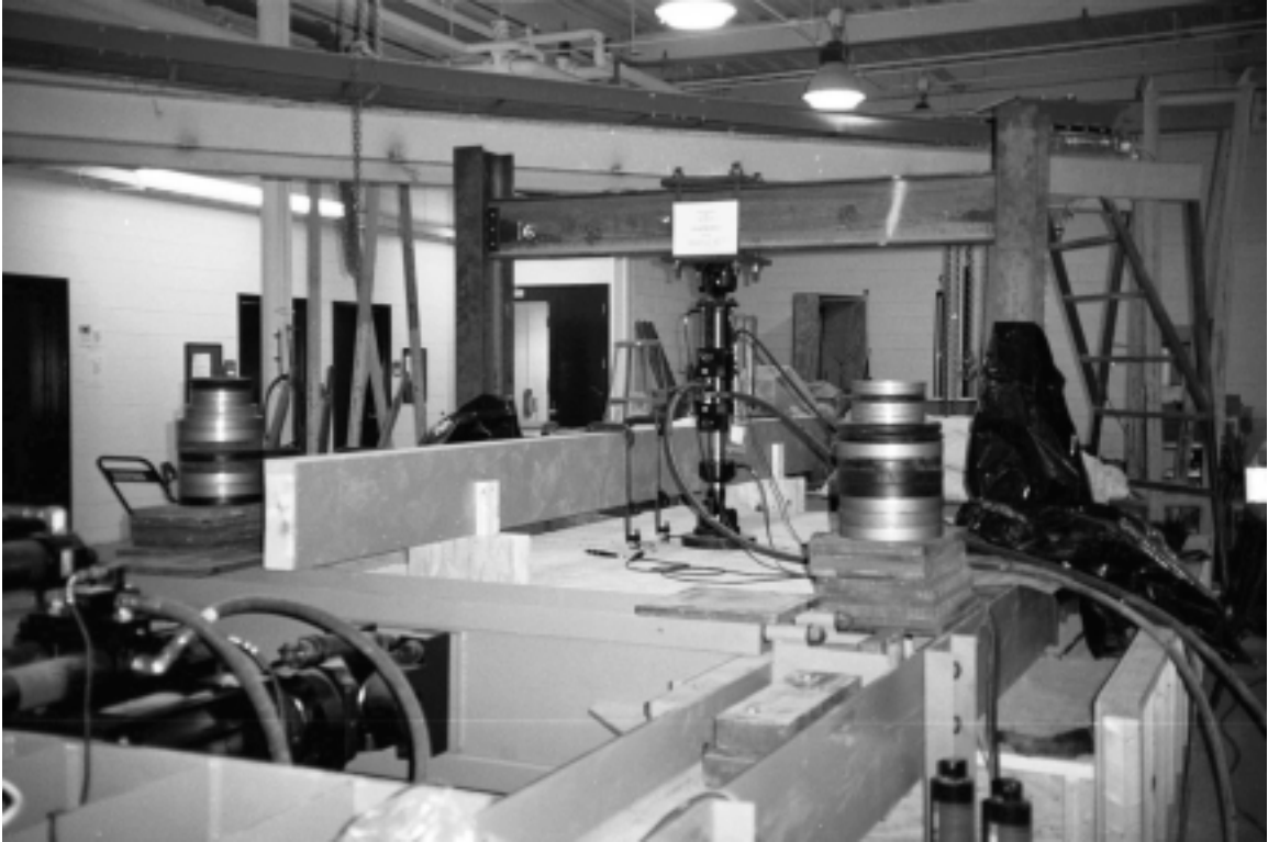
Figure 4.5 Overview of test set-up, reference beam
