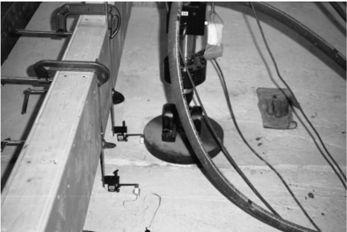
Figure 4.6 Overview of test set-up: loading plate, extensometers for measuring vertical deflections and location for measuring surface crack width is shown.
