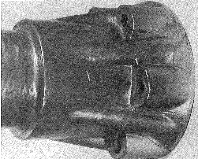
Figure 5. Typical failures of each of the two types of plastic fiberglass chord connections after ultimate tensile load tests, the chord-to-chord connection above and the diagonal-to-chord connection at right.
