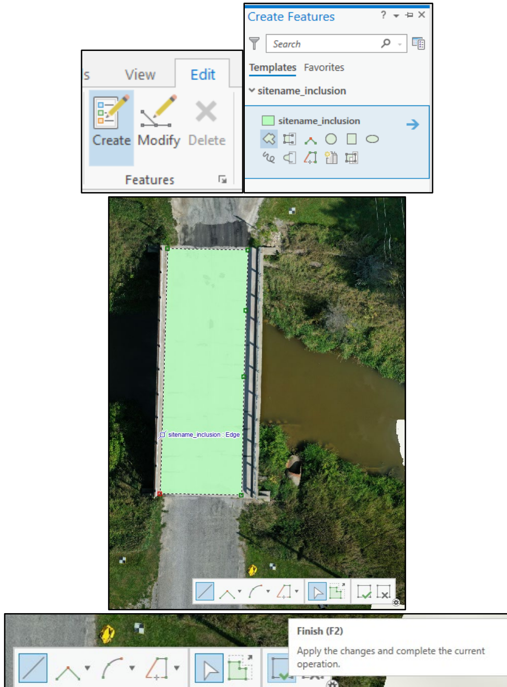
Figure 6.3.3: Drawing a polygon in ArcGIS Pro to set the analysis inclusion zone.
