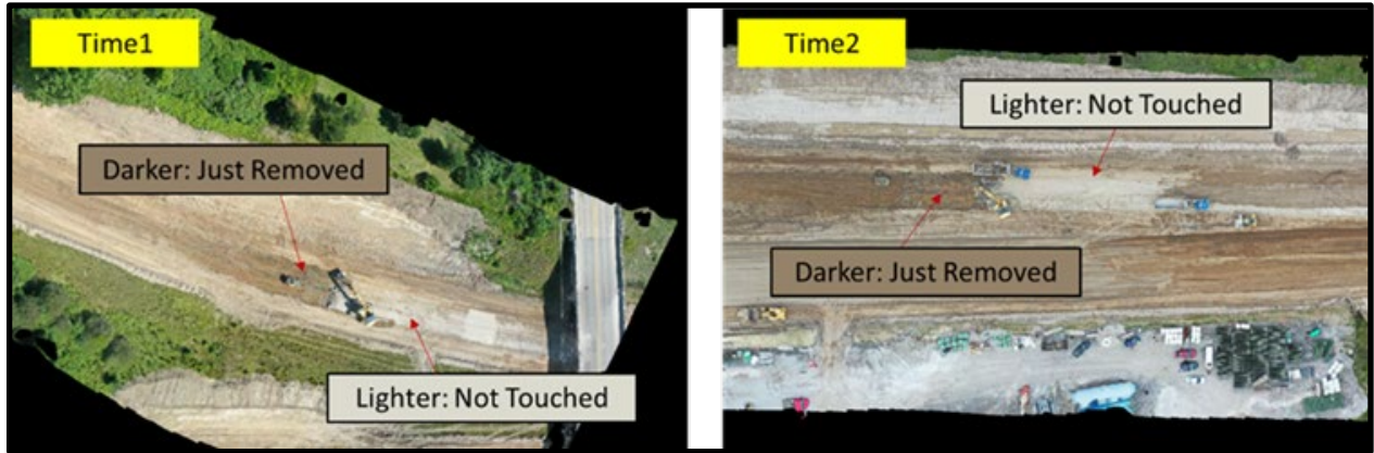
Figure 3.3.3: Image processing example one – MDOT I-496 Project (Samsami et al., 2021). Example image parameters used to identify disturbed vs. undisturbed areas during pavement removal.
