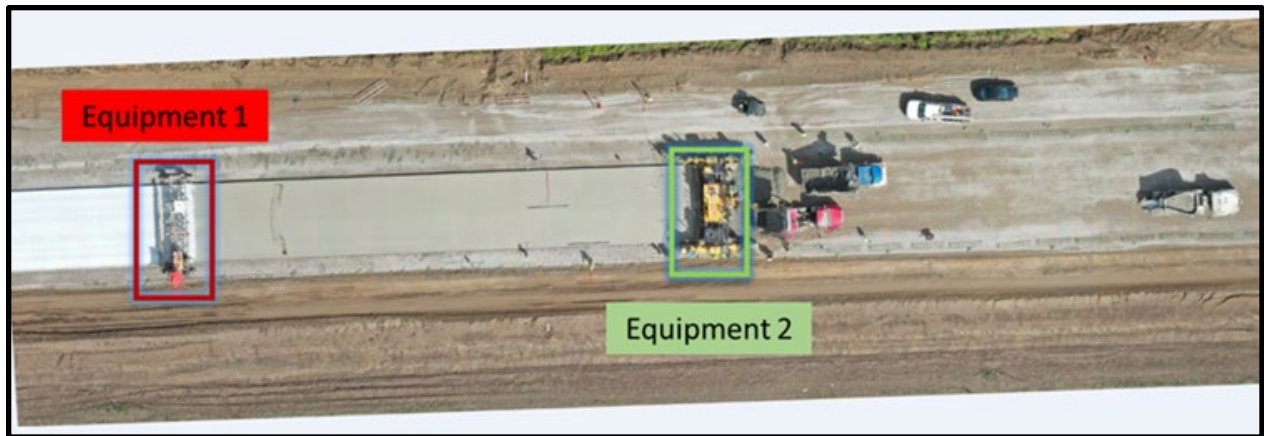
Figure 3.3.5: Image labeling example – MDOT I-496 Project (Samsami et al., 2021). Equipment can be identified in drone imagery/orthoimages using automated image processing packages available in MATLAB.
