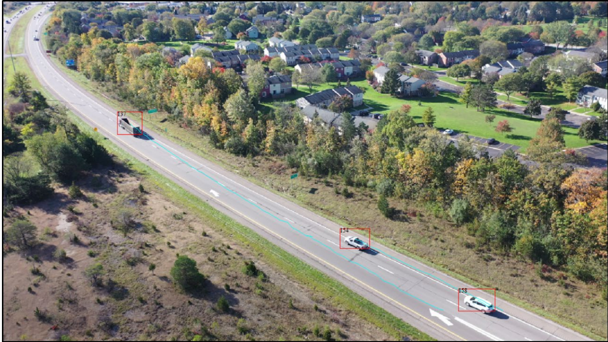
Figure 3.1.16: Automatic vehicle detection and tracking at US23/M14 weaving area.
