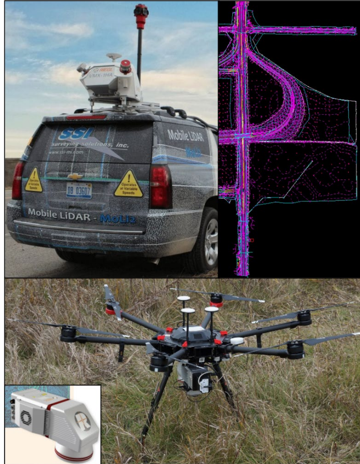
Figure 3.4.2: SSI’s MLS and UAS- based LiDAR systems (top left, bottom-right), and example DGN file containing traditional survey data for soft surfaces.
