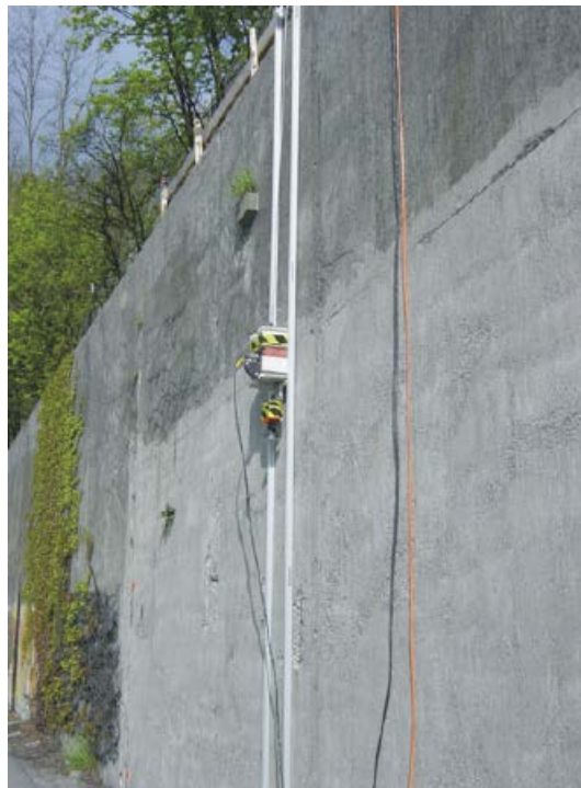
Figure 1.12. Semi-automated survey apparatus (from Hugenschmidt and Kalogeropoulos 2009)
