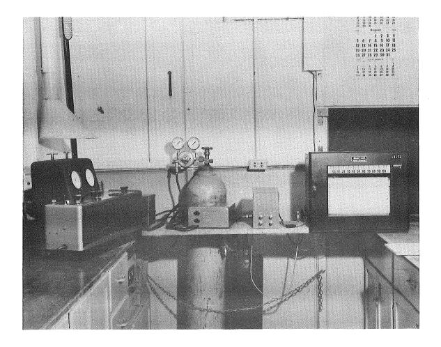
Figure 1. Recording Flame Photometer
