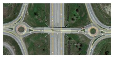
On-site observers found that the many trucks using this interchange at I-75 and M-81 in Saginaw County are able to maneuver through the roundabouts with relative ease. (Source: Google.)
