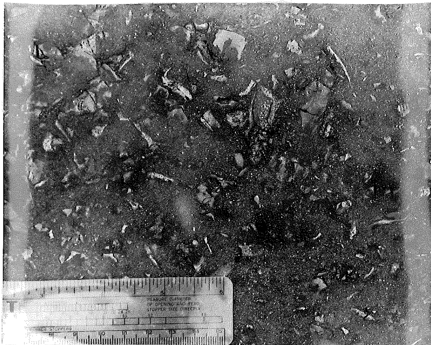
Figure 16. Wallace Limestone in Recap on US-10 north of Flint, Const. Proj. F 25-4, Cll. Shows condition on 2-23-49.
