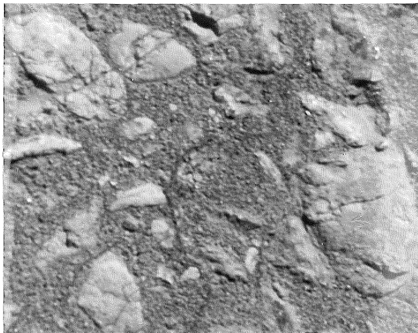
Figure 8. Sample of Bituminous Concrete Resurfacing from area on US-12 just east of Five Points, 3 miles east of Adamsville, Const. Proj. 14-15, C6, France Stone.
