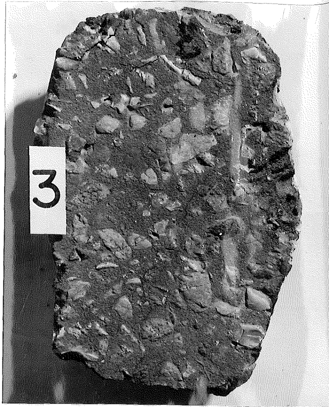
Figure 8. Sample of Bituminous Concrete Resurfacing from area on US-12 just east of Five Points, 3 miles east of Adamsville, Const. Proj. 14-15, C6, France Stone.
