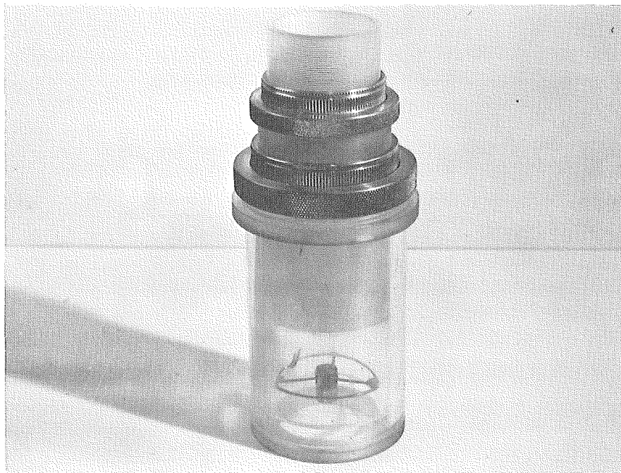
Figure 4. - Beta Gage showing source holder, plastic cylinders and brass friction rings comprising interior - assembled.
