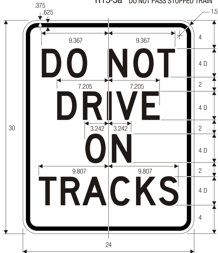
R15-6a DO NOT DRIVE ON TRACKS
