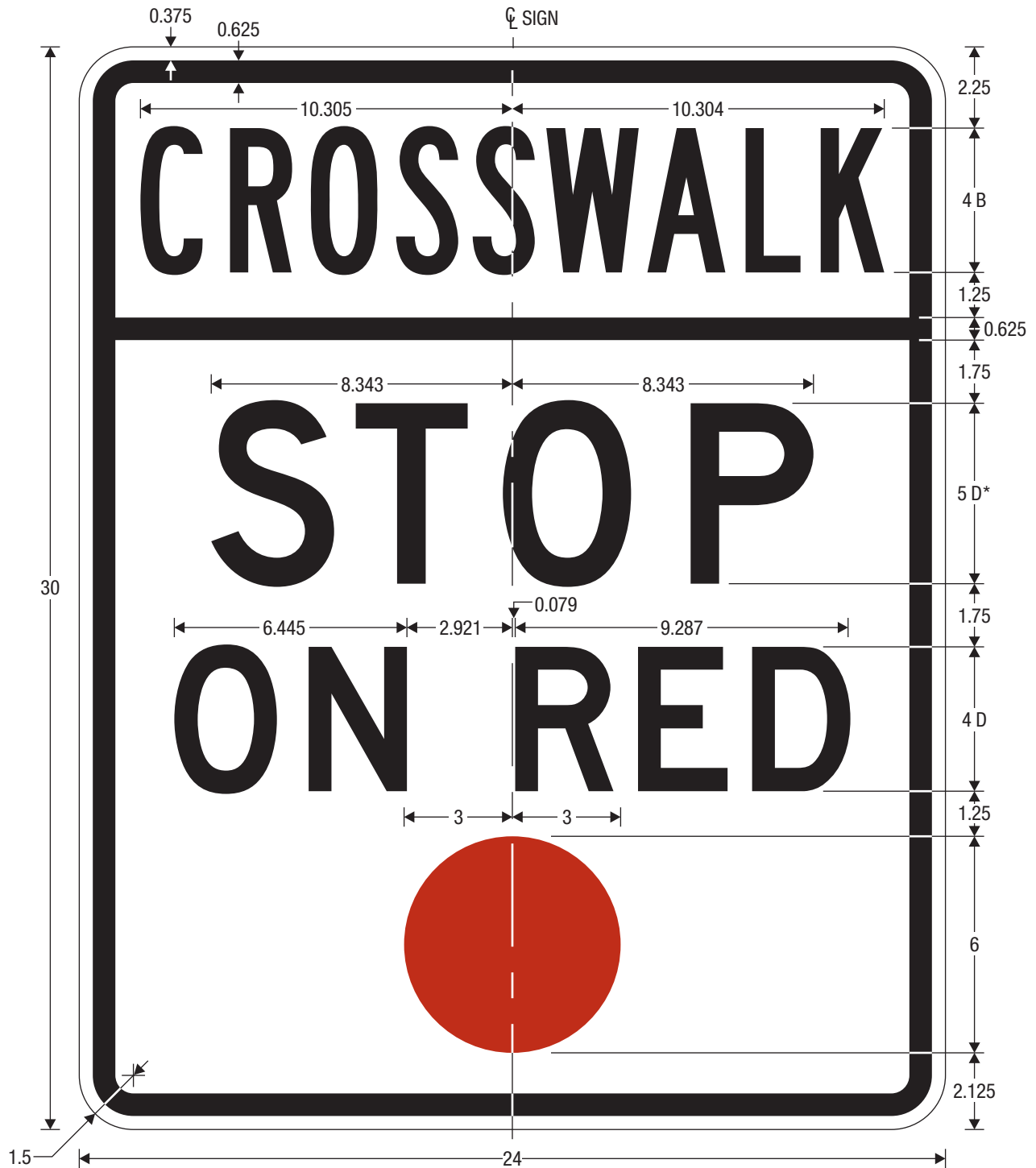
R10-23 CROSSWALK - STOP ON RED
