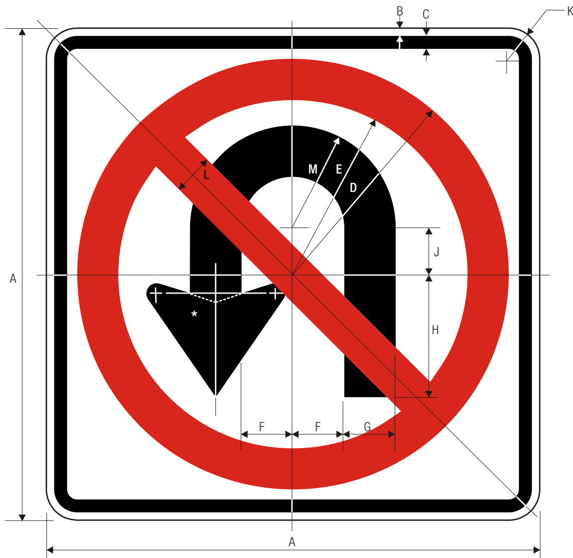
R3-4 U-TURN PROHIBITED
