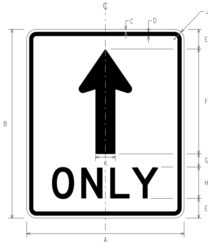
R3-5a OVERHEAD LANE USE SIGN (THRU ONLY)
