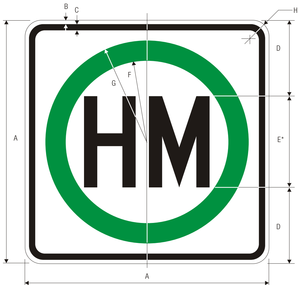
R14-2 HAZARDOUS MATERIAL
