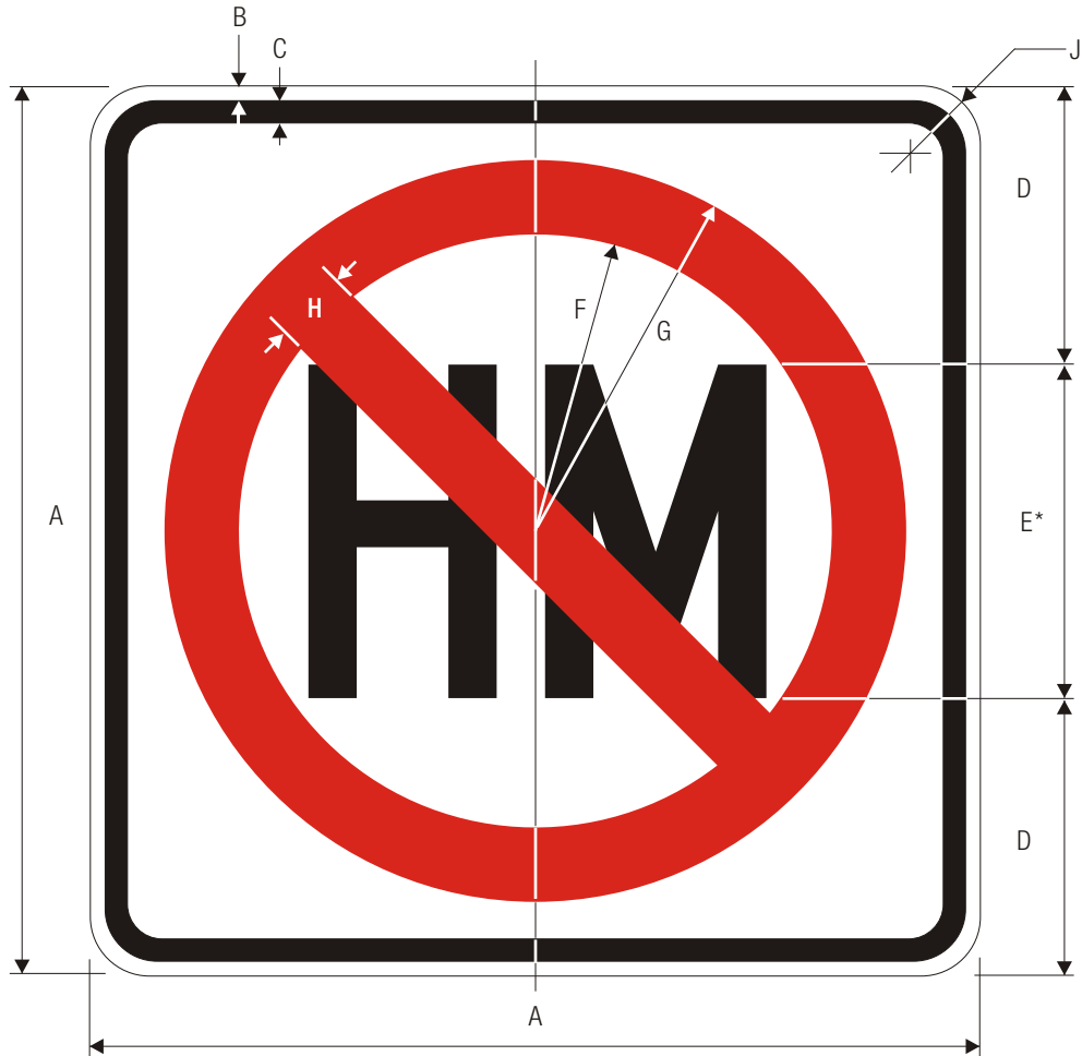
R14-3 HAZARDOUS MATERIAL
