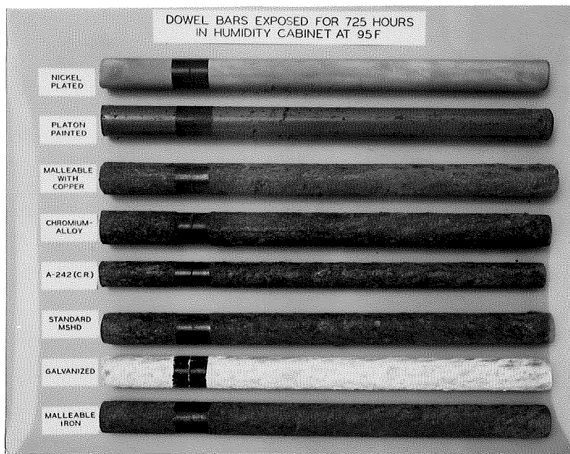
Figure 7. Condition of several dowel materials subjected to accelerated corrosion test.
